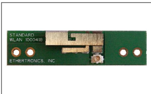
Ethertronics' Prestta series of Isolated Magnetic Dipole™ (IMD) stamped metal antennas address the challenges facing today's product designers. IMD's high performance and isolation characteristics offer better connectivity and minimal interference.
