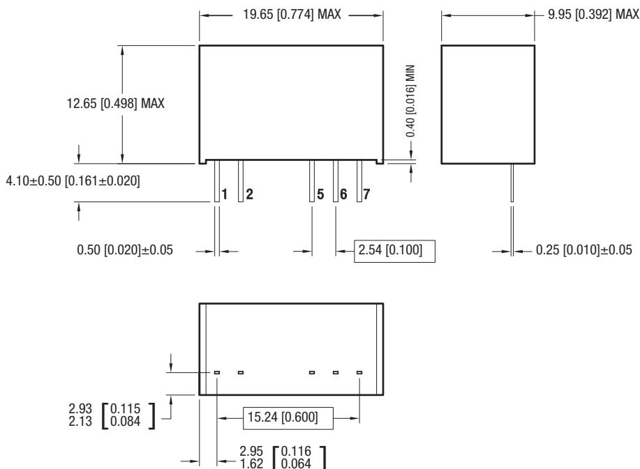
All dimensions in mm  $\pm 0.25$ mm (inches  $\pm 0.01$ ). All pins on a 2.54 (0.1) pitch and within  $\pm 0.25$  (0.01) of true position.
