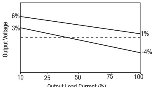
**NEGATIVE OUTPUT VOLTAGE TOLERANCE ENVELOPES**
