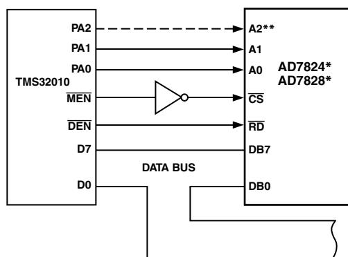
Figure 18. AD7824/AD7828-TMS32010 Interface
