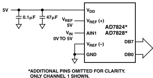
Figure 10. AD7824/AD7828 Unipolar 0 V to 5 V Operation
