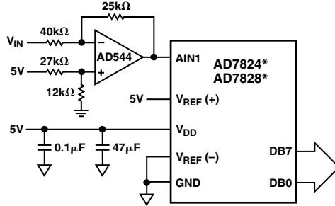
Figure 12. AD7824/AD7828 Bipolar  $\pm 4$  V Operation
