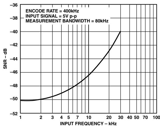
TPC 3. Signal Noise Ratio vs. Input Frequency
