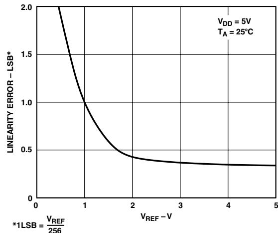
TPC 2. Accuracy vs.  $V_{REF}$  [ $V_{REF} = V_{REF}(+) - V_{REF}(-)$ ]
