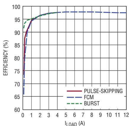
Figure 3. Measured Efficiency
