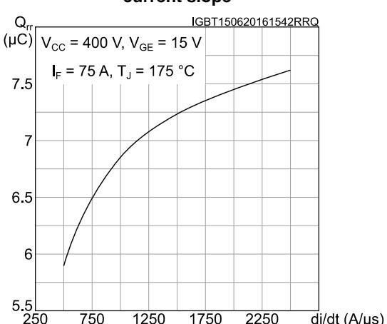
Figure 26: Reverse recovery energy vs. diode current slope
