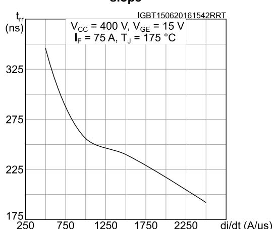
**Figure 25: Reverse recovery charge vs. diode current slope**
