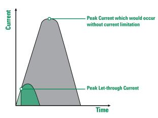
Figure 6 - Current limiting effect of fuses
