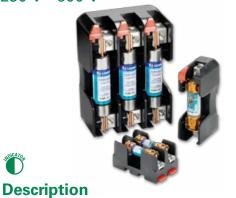
The Littelfuse Class H/K5 and R blocks offer many benefits such as indication, snap-to-release DIN rail mounting and universal mounting holes. Class H and Class R fuse blocks are dimensionally the same, but Class R blocks incorporate a rejection feature, which only allows Class R fuses to be inserted.
