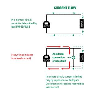
Figure 16 – Current Flow in Normal and Short Circuit Situations
