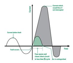
Figure 13 - Current-limiting Fuse
