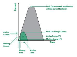
Figure 11 – Arcing and melting currents plus arcing, melting and clearing
