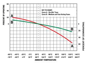
Figure 2 - Fuse Rerating Curve
