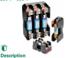
The Littelfuse Class H/K5 and R blocks offer many benefits such as indication, snap-to-release DIN rail mounting and universal mounting holes. Class H and Class R fuse blocks are dimensionally the same, but Class R blocks incorporate a rejection feature, which only allows Class R fuses to be inserted.
