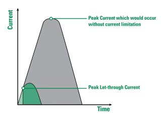
Figure 6 - Current limiting effect of fuses
