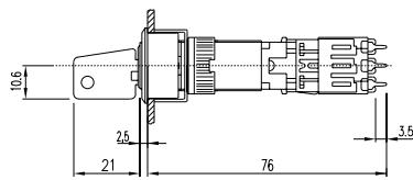
**51 keylock switch 2 positions for flush mounting 51 - 79 mm**
