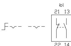
**37 selector switch 2 positions 45 - 70 mm, selector switch 2 positions for flush mounting 51 - 79 mm**
