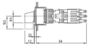
**56 selector switch 2 positions for flush mounting 51 - 79 mm**
