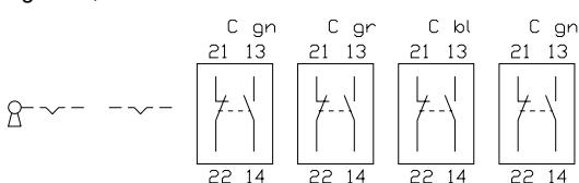
**29 keylock switch 2 positions 45 - 70 mm, keylock switch 2 positions for flush mounting 51 - 79 mm**
