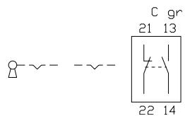
**25 keylock switch 2 positions 45 - 70 mm, keylock switch 2 positions for flush mounting 51 - 79 mm**
