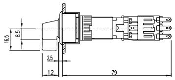
**58 protective cover for 35 mm, protective cover for illuminated-/pushbutton 55 - 70 mm**
