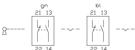
**36 selector switch 2 positions 45 - 70 mm, selector switch 2 positions for flush mounting 51 - 79 mm**
