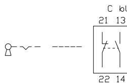
**22 keylock switch 2 positions 45 - 70 mm, keylock switch 2 positions for flush mounting 51 - 79 mm**
