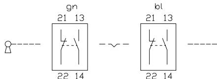
**34 keylock switch 3 positions 45 mm, keylock switch with 3 positions for flush mounting 51 - 54 mm**
