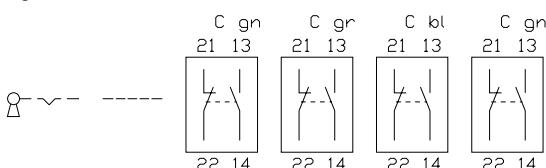
**30 keylock switch 2 positions 45 - 70 mm, keylock switch 2 positions for flush mounting 51 - 79 mm**
