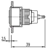
37 indicator for flush mounting 39 - 79 mm
