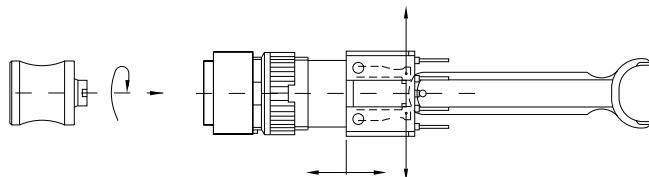
Push-pull knob can be mounted in only one position. Zero position
