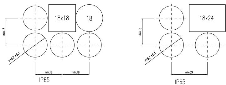
**3 indicator 30 - 70 mm, illuminated-/pushbutton 55 - 70 mm**
