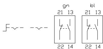
**39 selector switch 2 positions 45 - 70 mm, selector switch 2 positions for flush mounting 51 - 79 mm**
