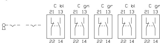
**31 keylock switch 2 positions 45 - 70 mm, keylock switch 2 positions for flush mounting 51 - 79 mm**
