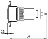
38 indicator for flush mounting 39 - 79 mm, buzzer for flush mounting 39 - 64 mm
