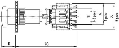
**21 keylock switch 2 positions 45 - 70 mm, keylock switch 3 positions 45 mm**
