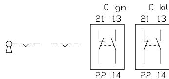
**23 keylock switch 2 positions 45 - 70 mm, keylock switch 2 positions for flush mounting 51 - 79 mm**
