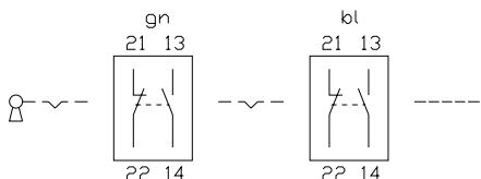
**35 keylock switch 3 positions 45 mm, keylock switch with 3 positions for flush mounting 51 - 54 mm**
