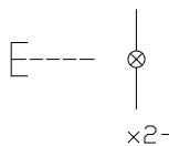
3 pushbutton-/illuminated pushbutton actuator 35 mm
