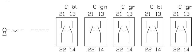
**32 keylock switch 3 positions 45 mm, keylock switch with 3 positions for flush mounting 51 - 54 mm**
