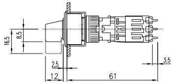
**55 selector switch 2 positions for flush mounting 51 - 79 mm**
