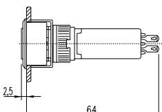
40 indicator for flush mounting 39 - 79 mm
