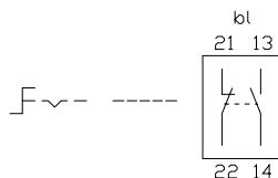
**38 selector switch 2 positions 45 - 70 mm, selector switch 2 positions for flush mounting 51 - 79 mm**
