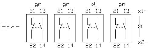
**8 illuminated-/pushbutton 55 - 70 mm, pushbutton-/illuminated pushbutton for flush mounting 61 - 79 mm**
