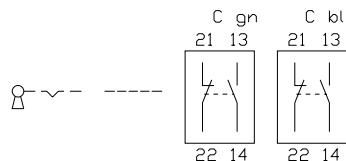
**24 keylock switch 2 positions 45 - 70 mm, keylock switch 2 positions for flush mounting 51 - 79 mm**
