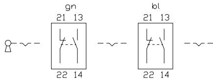
**33 keylock switch 3 positions 45 mm, keylock switch with 3 positions for flush mounting 51 - 54 mm**
