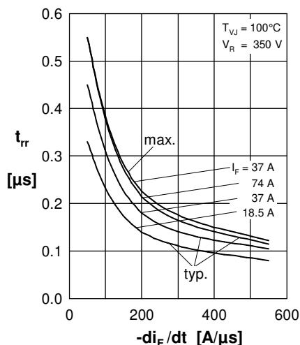
Fig. 5 Typ. recovery time  $t_{rr}$  versus  $-di_F/dt$
