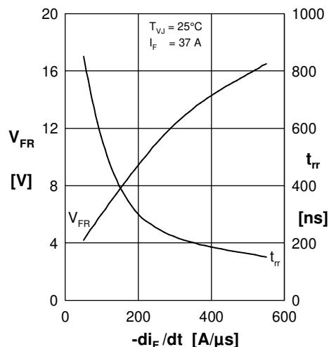
Fig. 6 Typ. peak forward voltage  $V_{FR}$  and  $t_{rr}$  versus  $-di_F/dt$
