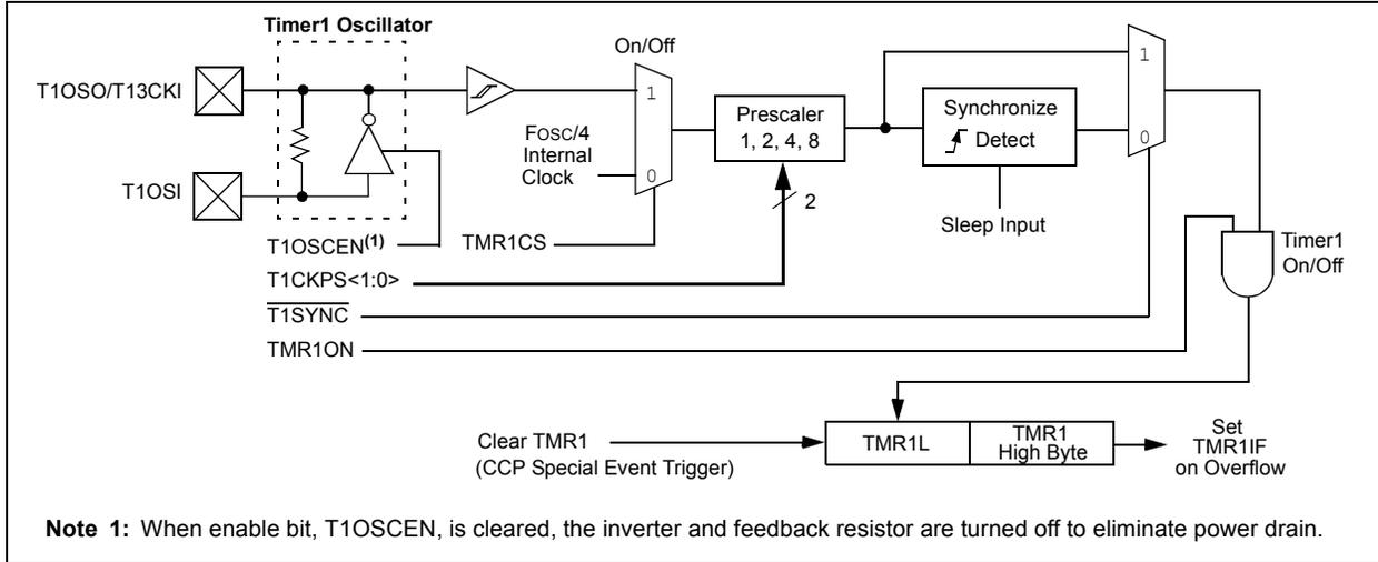
**FIGURE 13-2: TIMER1 BLOCK DIAGRAM (16-BIT READ/WRITE MODE)**
