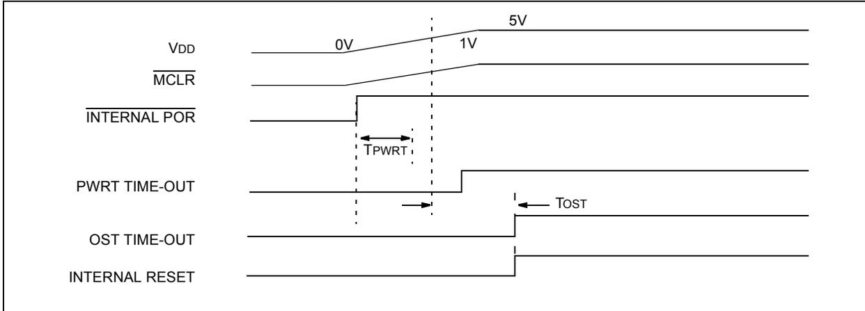
**FIGURE 5-7: TIME-OUT SEQUENCE ON POR W/PLL ENABLED ( $\overline{\text{MCLR}}$  TIED TO  $V_{DD}$ )**
