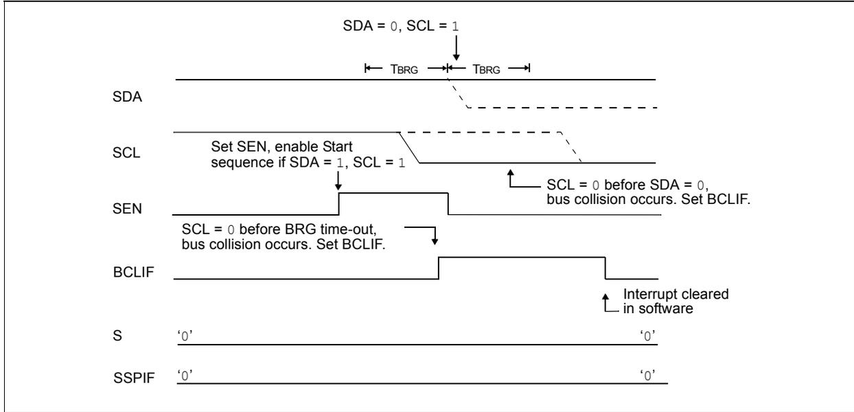
**FIGURE 18-28: BRG RESET DUE TO SDA ARBITRATION DURING START CONDITION**
