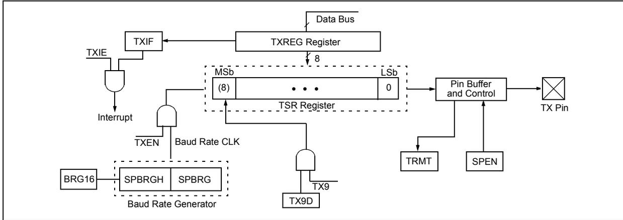
**FIGURE 19-4: ASYNCHRONOUS TRANSMISSION**
