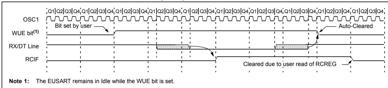
**FIGURE 19-9: AUTO-WAKE-UP BIT (WUE) TIMINGS DURING SLEEP**
