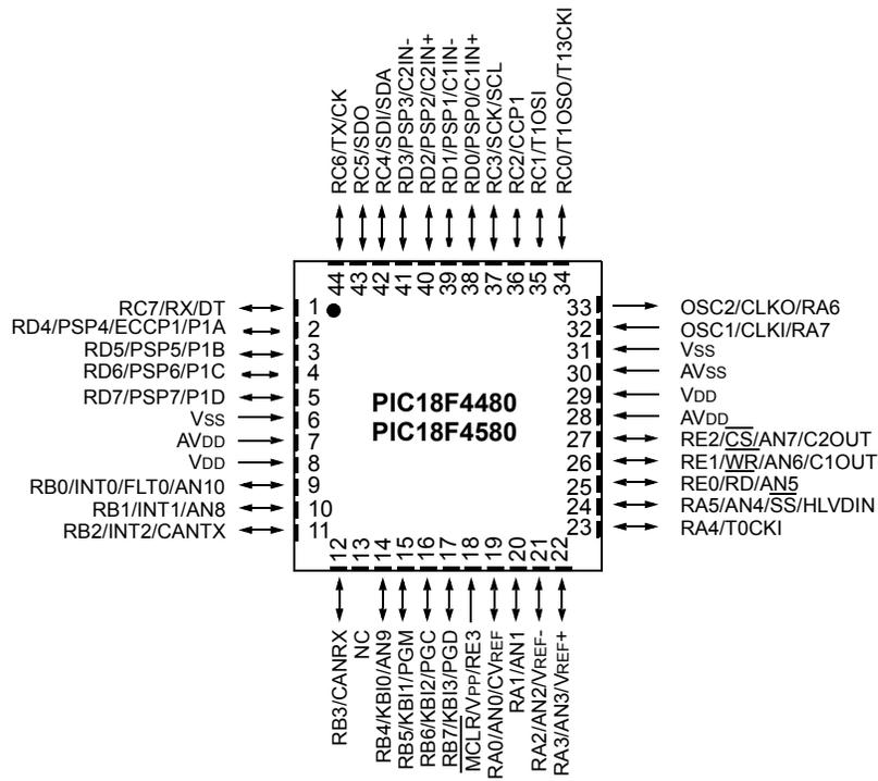
**Note 1:** For the QFN package, it is recommended that the bottom pad be connected to V<sub>SS</sub>.
