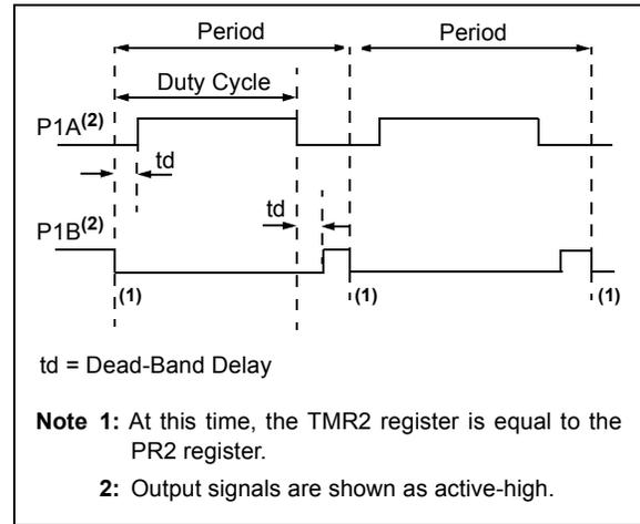
**FIGURE 17-5: EXAMPLES OF HALF-BRIDGE OUTPUT MODE APPLICATIONS**
