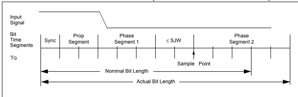
**FIGURE 24-7: SHORTENING A BIT PERIOD (SUBTRACTING SJW FROM PHASE SEGMENT 2)**
