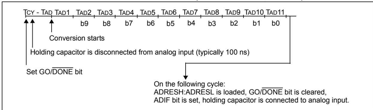
**FIGURE 20-4: A/D CONVERSION TAD CYCLES ( $\text{ACQT}<2:0> = 010, \text{TACQ} = 4 \text{TAD}$ )**
