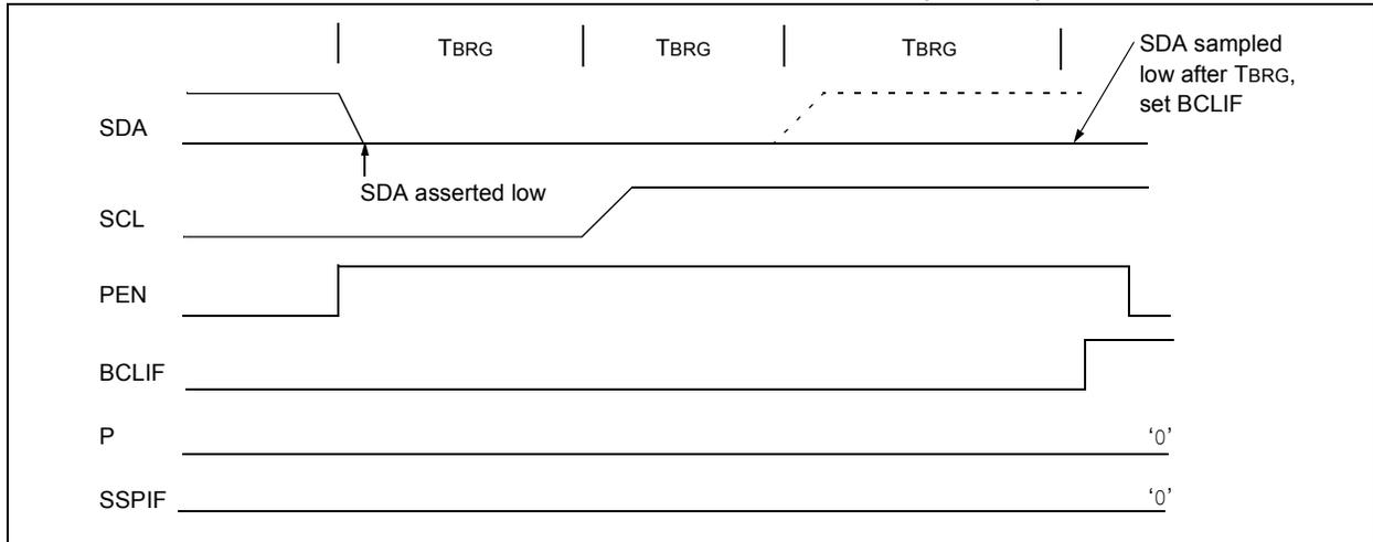
**FIGURE 18-32: BUS COLLISION DURING A STOP CONDITION (CASE 2)**
