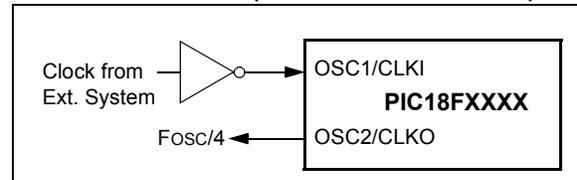
The ECIO Oscillator mode functions like the EC mode, except that the OSC2 pin becomes an additional general purpose I/O pin. The I/O pin becomes bit 6 of PORTA (RA6). Figure 3-4 shows the pin connections for the ECIO Oscillator mode.
