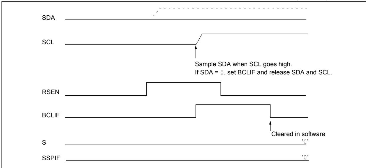
**FIGURE 18-30: BUS COLLISION DURING REPEATED START CONDITION (CASE 2)**
