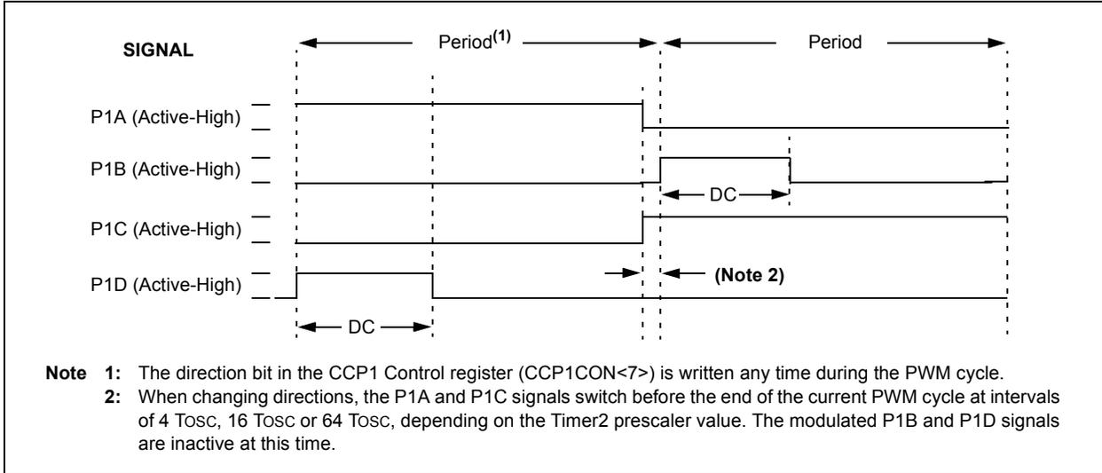
**FIGURE 17-9: PWM DIRECTION CHANGE AT NEAR 100% DUTY CYCLE**
