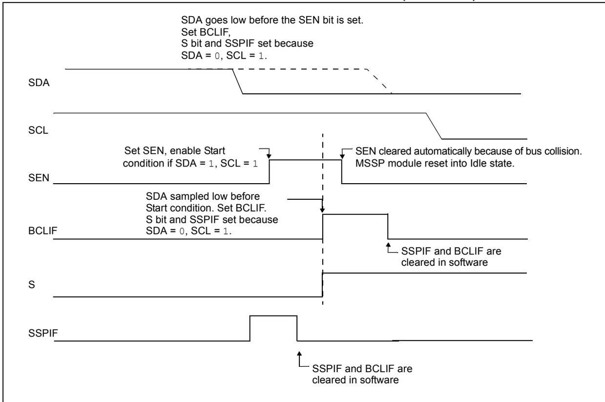
**FIGURE 18-27: BUS COLLISION DURING START CONDITION (SCL = 0)**
