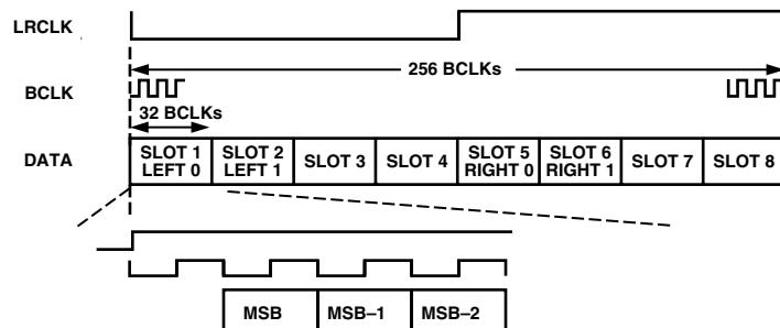
Figure 5. ADC Packed Mode 256
