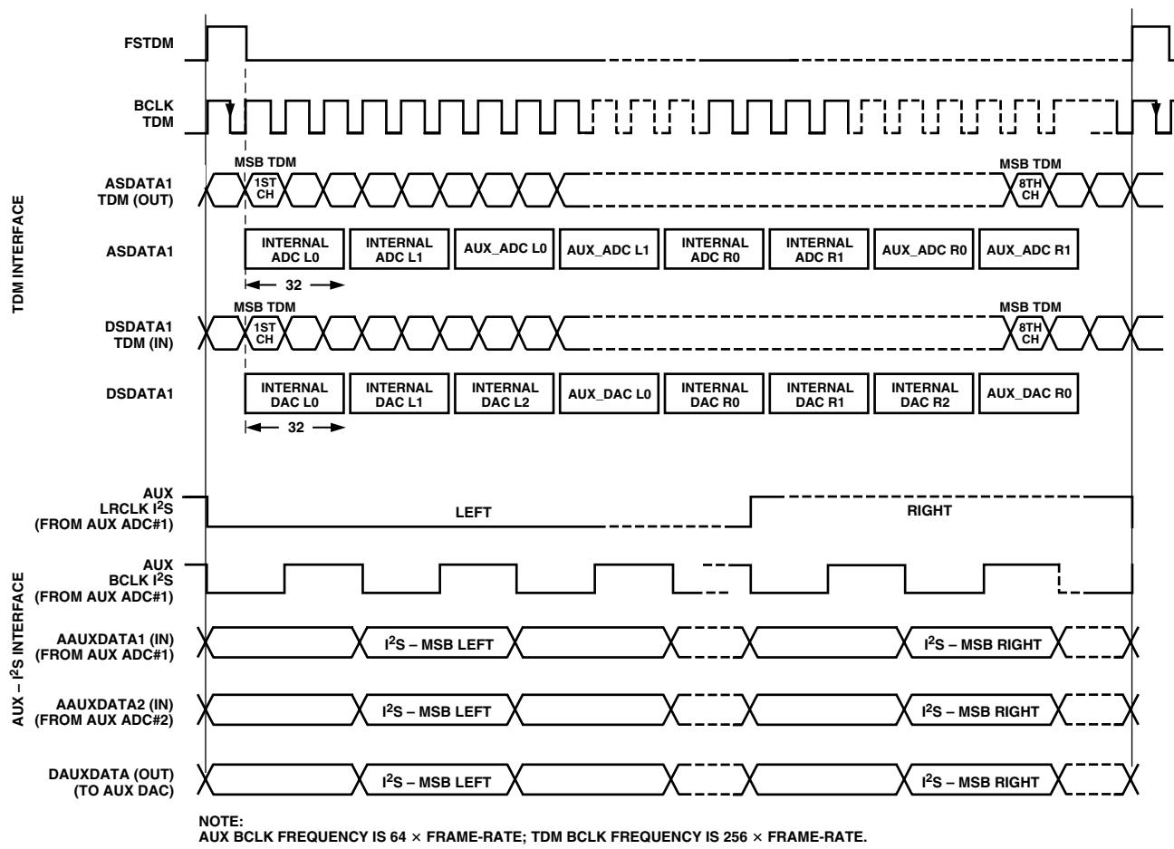
Figure 8. AUX-Mode Timing
