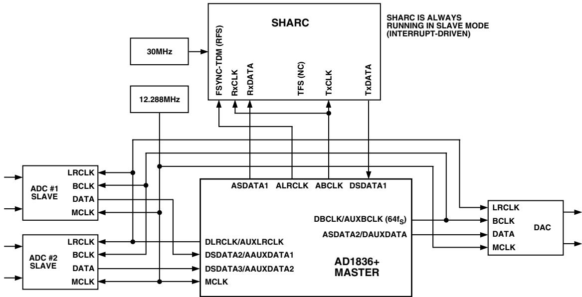
Figure 9. AUX-Mode Connection to SHARC (Master Mode)
