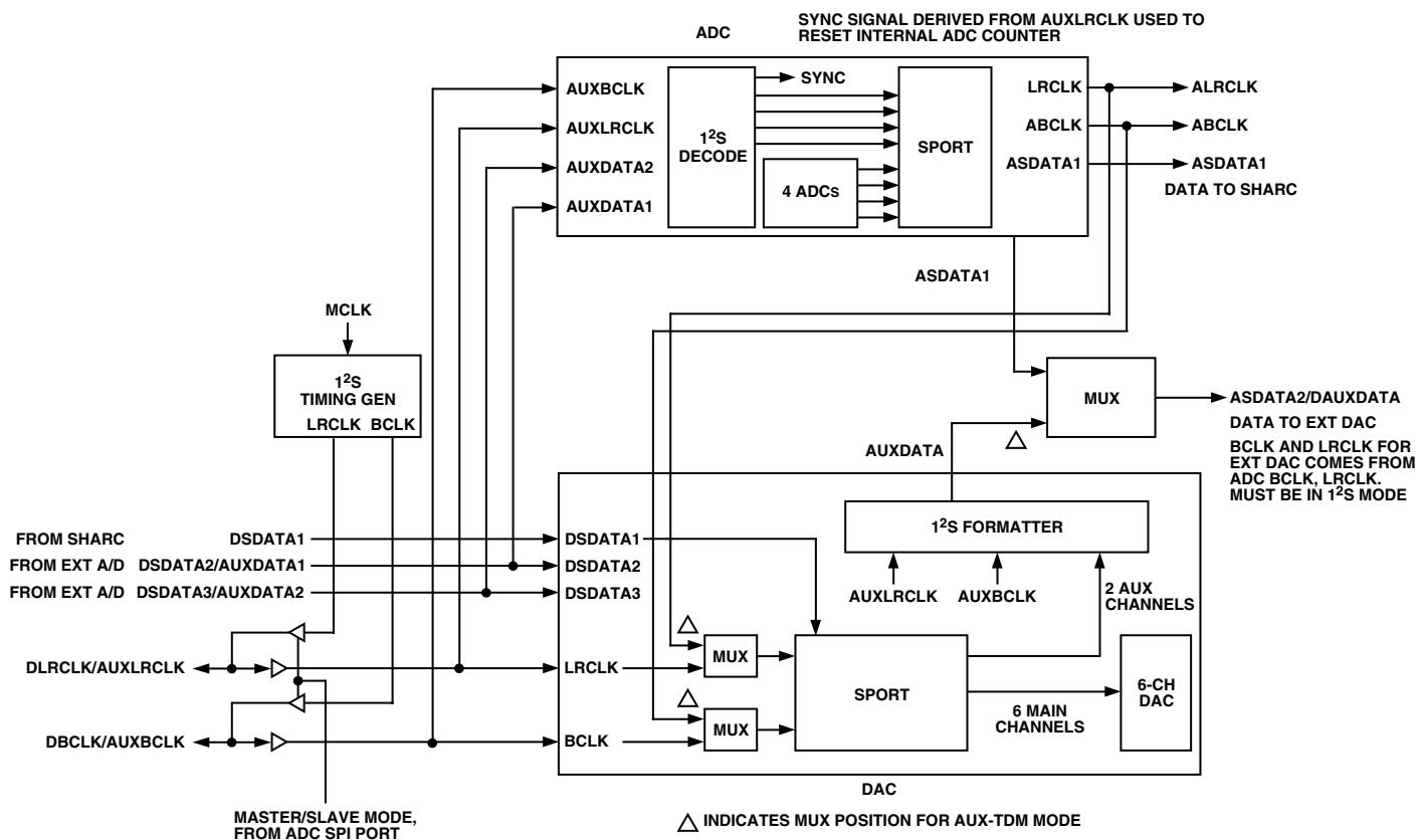
*Figure 11. Extended TDM Mode Internal Flow Diagram*
