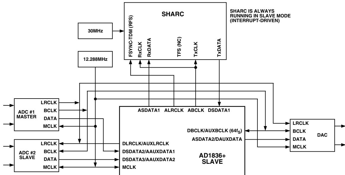
Figure 10. AUX-Mode Connection to SHARC (Slave Mode)
