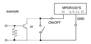
.... Output Voltage = ON .... Output Voltage = OFF
