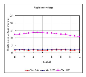
Fig. 12-3-6. Ripple Voltage v.s. Output Current
