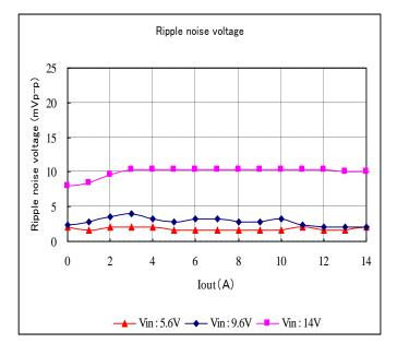
Fig. 12-3-15. Ripple Voltage v.s. Output Current
