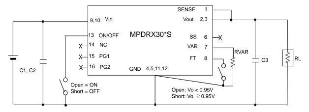
$\begin{array}{ll} \text{C1,C2}: 10\mu\text{F}\big/25\text{V} & \text{(Ceramic Capacitor)} \\ \text{C3}: 100\mu\text{F}\big/6.3\text{V} & \text{(Ceramic Capacitor)} \end{array}$
