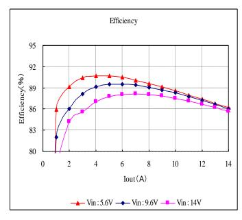
Fig. 12-3-8. Efficiency v.s. Output Current
