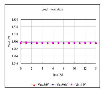
Fig. 12-3-7. Output Voltage v.s. Output Current
