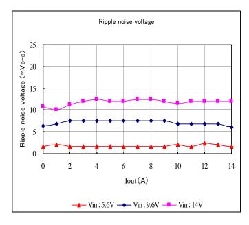
Fig. 12-3-18. Ripple Voltage v.s. Output Current
