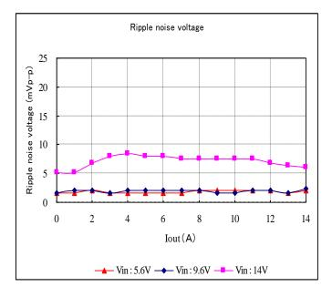
Fig. 12-3-12. Ripple Voltage v.s. Output Current
