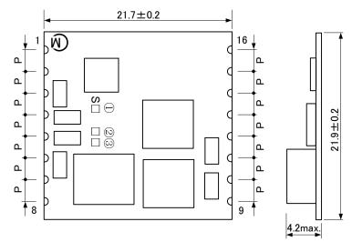
$P=2.54 \pm 0.2 mm$ Tolerance is not accumulated.
