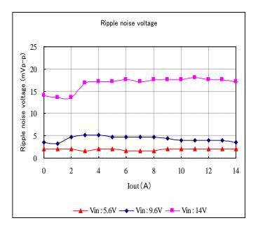
Fig. 12-3-9. Ripple Voltage v.s. Output Current
