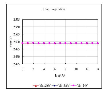
Fig. 12-3-4. Output Voltage v.s. Output Current
