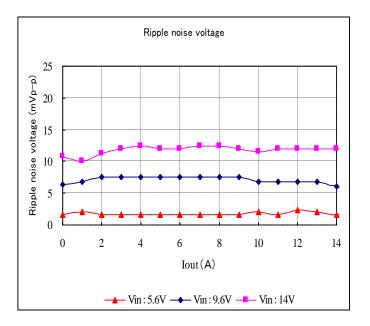
Fig. 12-3-18. Ripple Voltage v.s. Output Current
