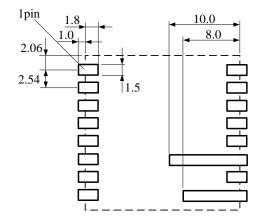
There are wiring coppers or through-hole via at the bottom side of the DC-DC converter. When you design your PCBs, please be careful not to short the circuit of the DC-DC converter or PCBs.
