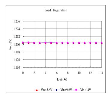
Fig. 12-3-13. Output Voltage v.s. Output Current
