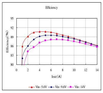
Fig. 12-3-8. Efficiency v.s. Output Current
