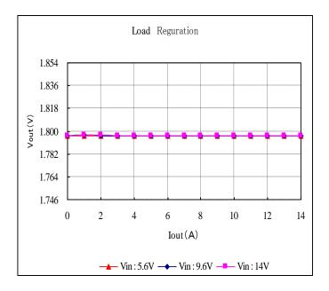
Fig. 12-3-7. Output Voltage v.s. Output Current
