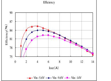
Fig. 12-3-17. Efficiency v.s. Output Current
