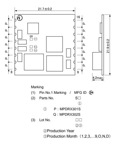
P=2.54 ±0.2mm Tolerance is not accumulated.
