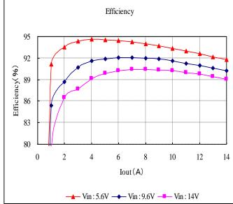
Fig. 12-3-2. Efficiency v.s. Output Current
