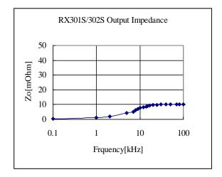
Fig. 12-2-1. Output Impedance of MPDRX301S/302S
