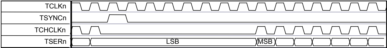
Figure 11-31. E1 Transmit-Side TCHCLKn Gapped Mode During Channel 1
