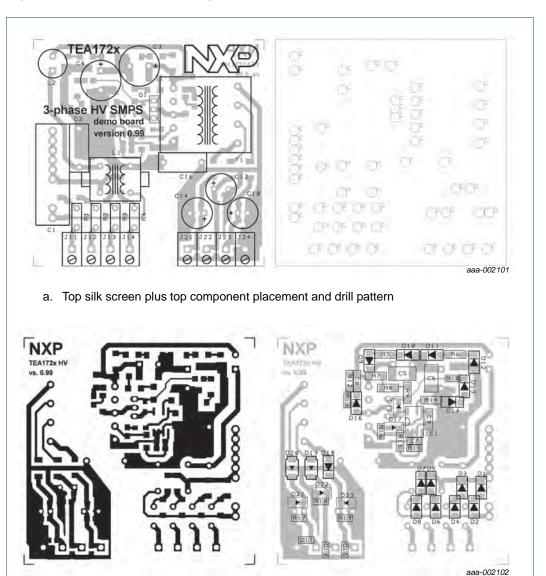
b. Bottom copper and bottom silk screen plus component placement
