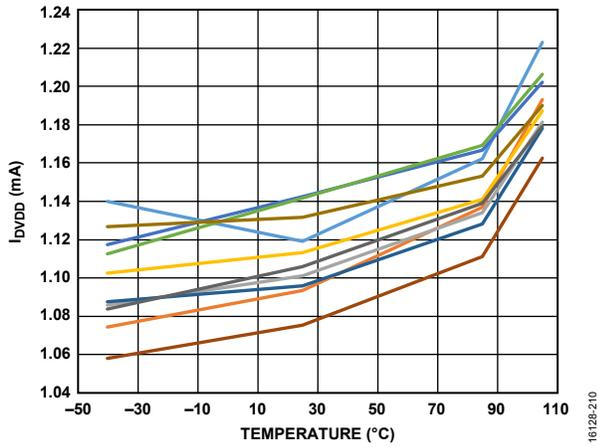
Figure 68.  $I_{DVDD}$  vs. Temperature for Ten AD5770R Devices
