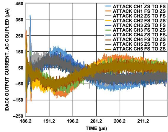
Figure 55. DAC to DAC Crosstalk (Victim Channel Zero)
