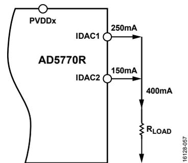
Figure 77. Increasing the Current Range by Summing Channels
