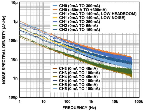
Figure 51. Output NSD vs. Frequency (All Ranges)
