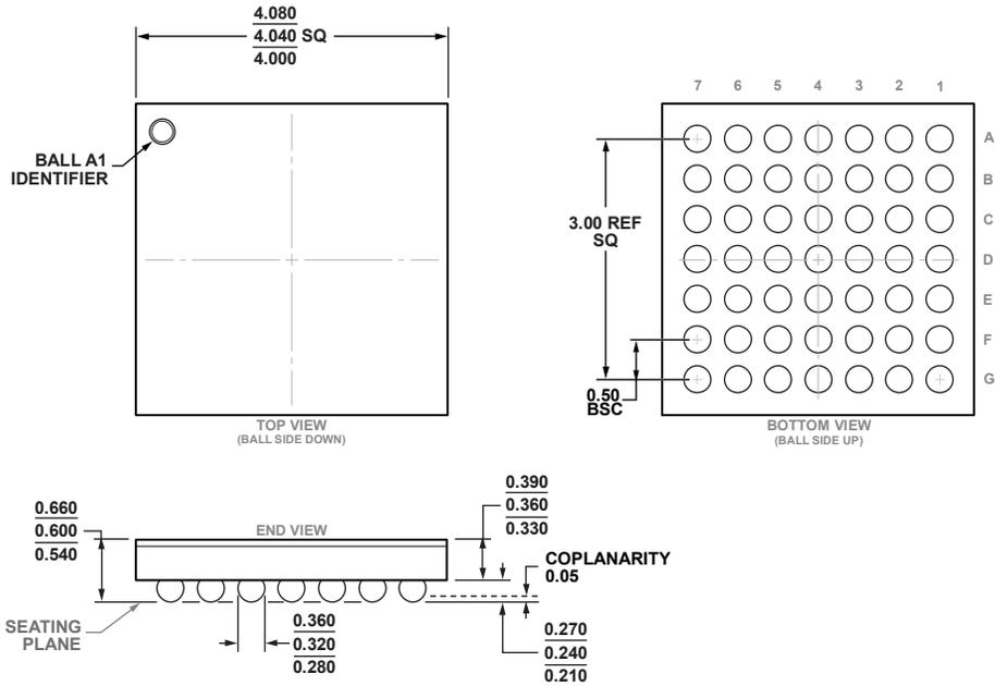
Figure 78. 49-Ball Wafer Level Chip Scale Package [WLCSP]
