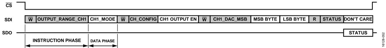
Figure 74. SPI Transaction in Single Instruction Mode
