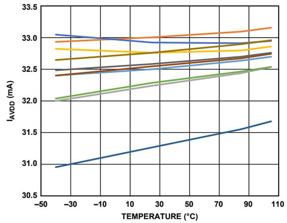
Figure 67.  $I_{AVDD}$  vs. Temperature for Ten AD5770R Devices
