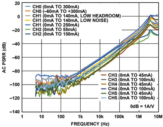
Figure 48. AC PSRR vs. Frequency (All Ranges)
