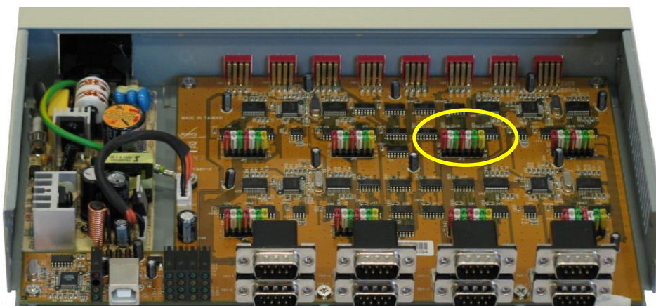
Figure 8 - ES-U-3008-RM has a set of jumpers for each port (one set circled)
