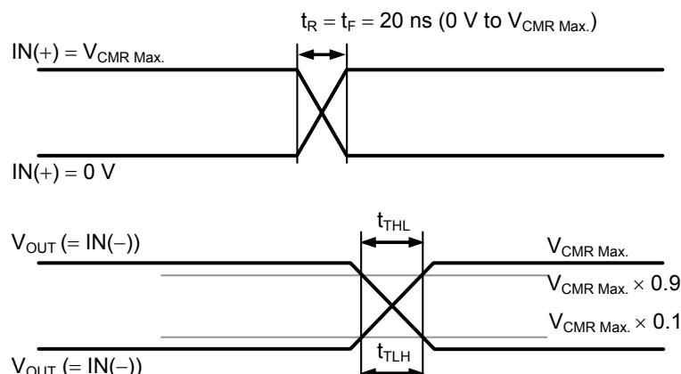
$$SR = \frac{V_{CMR\ Max.} \times 0.8}{t_{TLH}}$$
