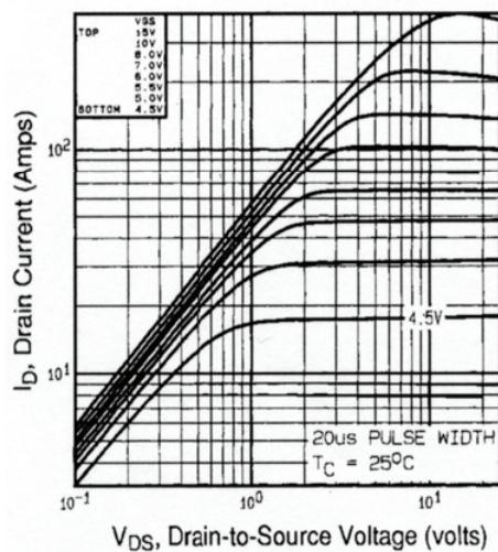
**Fig. 1 - Typical Output Characteristics,  $T_C = 25\text{ }^\circ\text{C}$**
