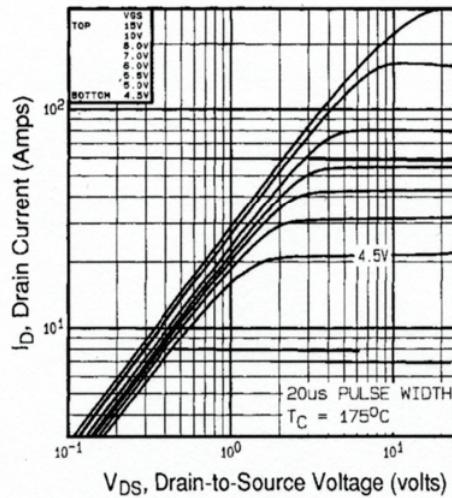
**Fig. 2 - Typical Output Characteristics,  $T_C = 175\text{ }^\circ\text{C}$**
