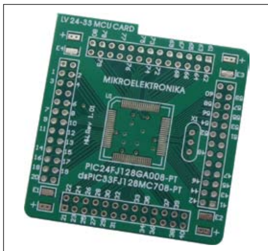
Figure 8: Empty MCU card MCU Card 3
