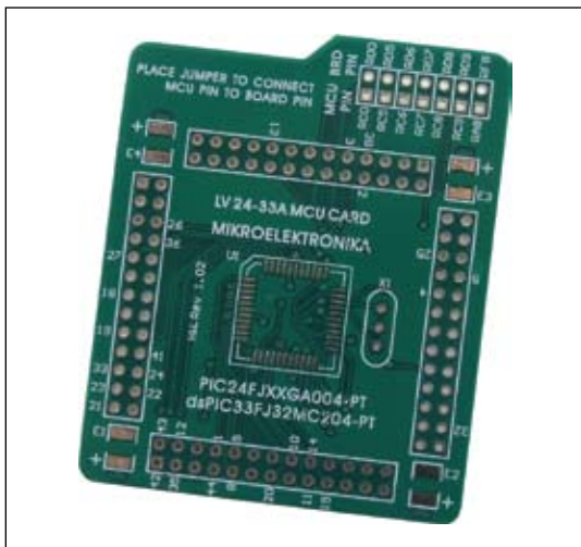
Figure 35: Empty MCU card MCU Card 12
