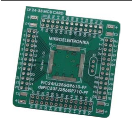
Figure 23: Empty MCU card MCU Card 8
