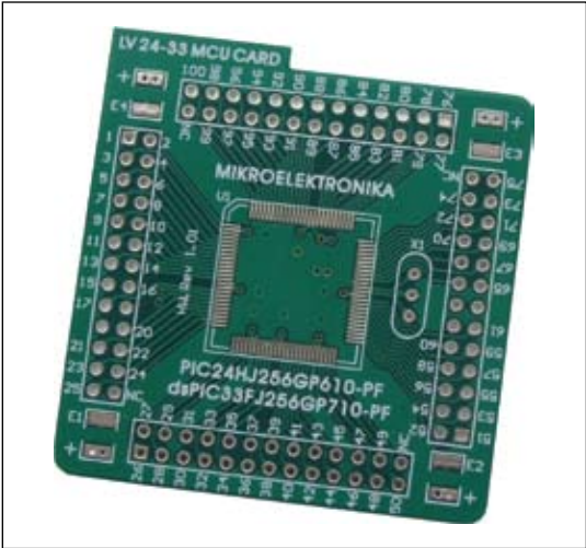
Figure 23: Empty MCU card MCU Card 8
