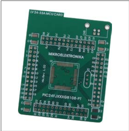
Figure 41: Empty MCU card MCU Card 14
