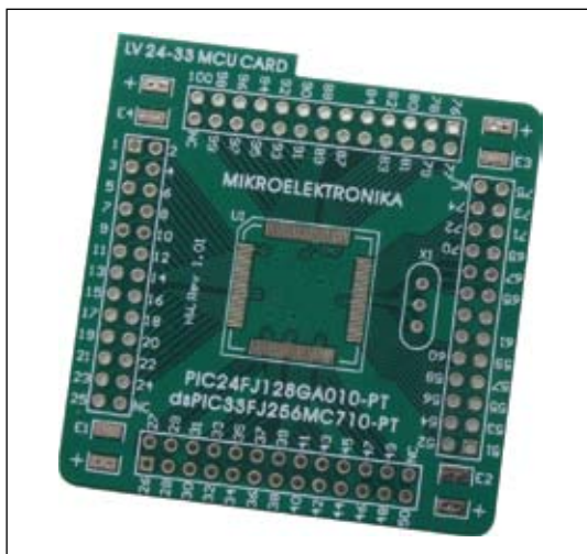
Figure 14: Empty MCU card MCU Card 5
