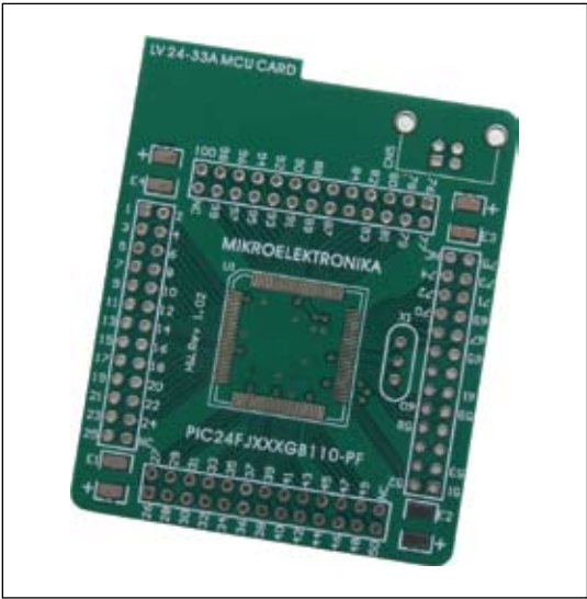
Figure 47: Empty MCU card MCU Card 16
