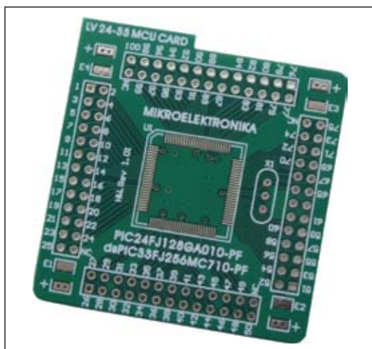
Figure 20: Empty MCU card MCU Card 7
