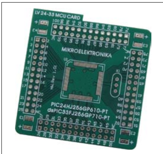
Figure 17: Empty MCU card MCU Card 6
