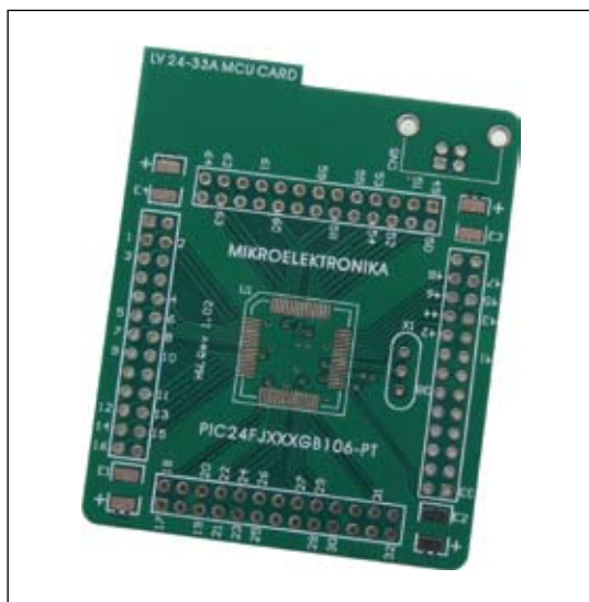
Figure 38: Empty MCU card MCU Card 13
