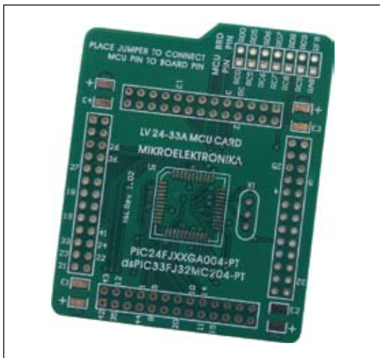
Figure 35: Empty MCU card MCU Card 12
