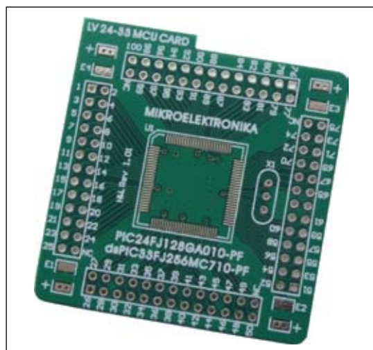
Figure 20: Empty MCU card MCU Card 7
