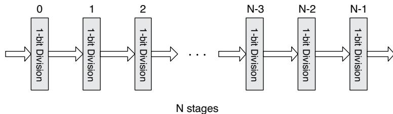
The Divider IP core uses a non-restoring division algorithm to implement the integer division operation.
