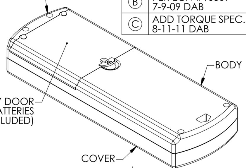
BATTERY DOOR HOLDS (4) 'AA' BATTERIES (CONTACT KIT IS INCLUDED)
