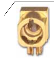
90 Degree receptacle mated to plug
