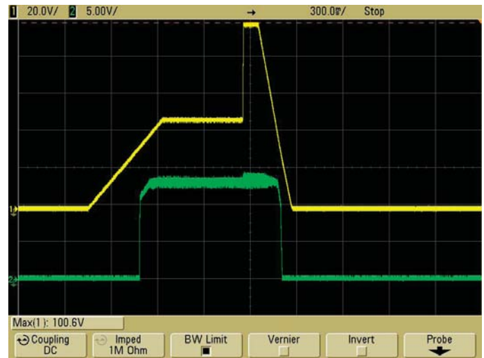
Figure 4. Test Waveform with Feedback Loop Open
