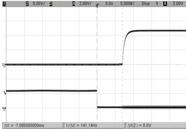
On/Off Enable start up (Vin=48V, Iout=20A, Cload=4700uf, Ta=+25°C) Ch2=Vout, Ch4=Enable
