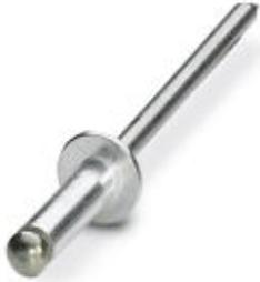
Blind rivets, Ø 4.8 mm, 12 mm sleeve length, aluminum sleeve, zinc-plated steel pin, flat head, standard version similar to DIN 7337 A
