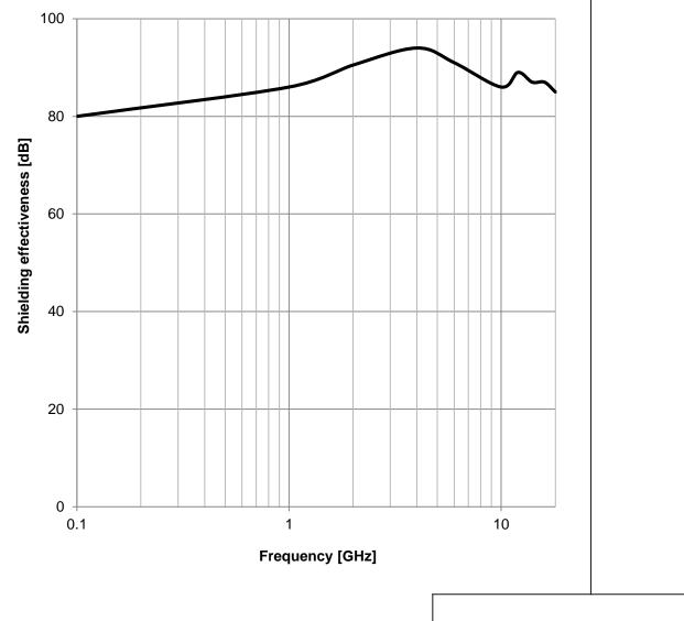
CHECKED REVISION DATE (YYYY-MM-DD) GENERAL TOLERANCE PROJECTION METHOD JoV 005.002 2019-01-01 DIN ISO 2768-1m DESCRIPTION **WE-LT Conductive Shielding** Würth Elektronik eiSos GmbH & Co. KG Gasket ORDER CODE EMC & Inductive Solutions Max-Eyth-Str. 1 3091010 74638 Waldenburg Germany SIZE/TYPE STATUS Tel. +49 (0) 79 42 945 - 0 www.we-online.com BUSINESS UNIT PAGE WÜRTH ELEKTRONIK 2/3 C-Profile eiSos Valid eiSos@we-online.com
