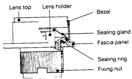
The first time the button is pressed, the gland is forced into its groove and becomes effective
