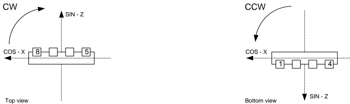
Figure 7: X/Z Magnetic Axis
