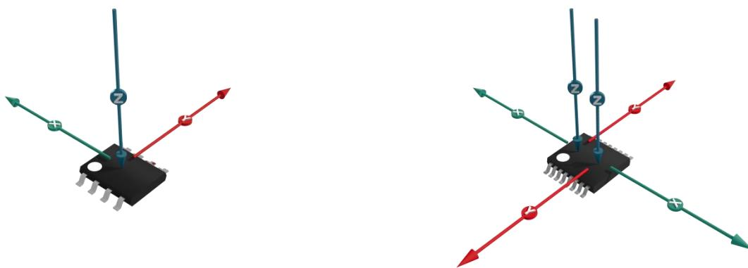
*Figure 5: Axis configuration*
