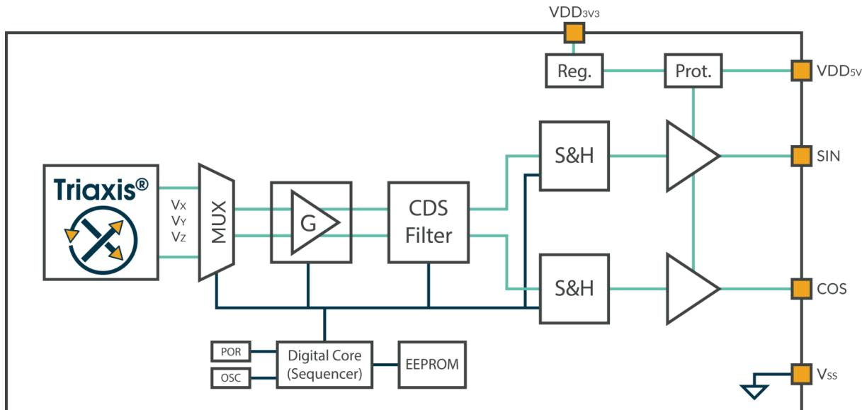
Figure 3: Functional Diagram
