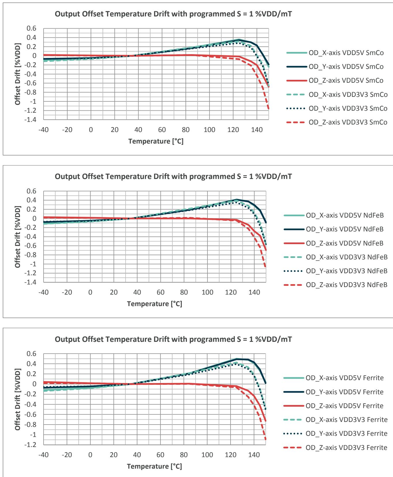
Figure 10: Output Offset Temperature Drift per Magnet Type
