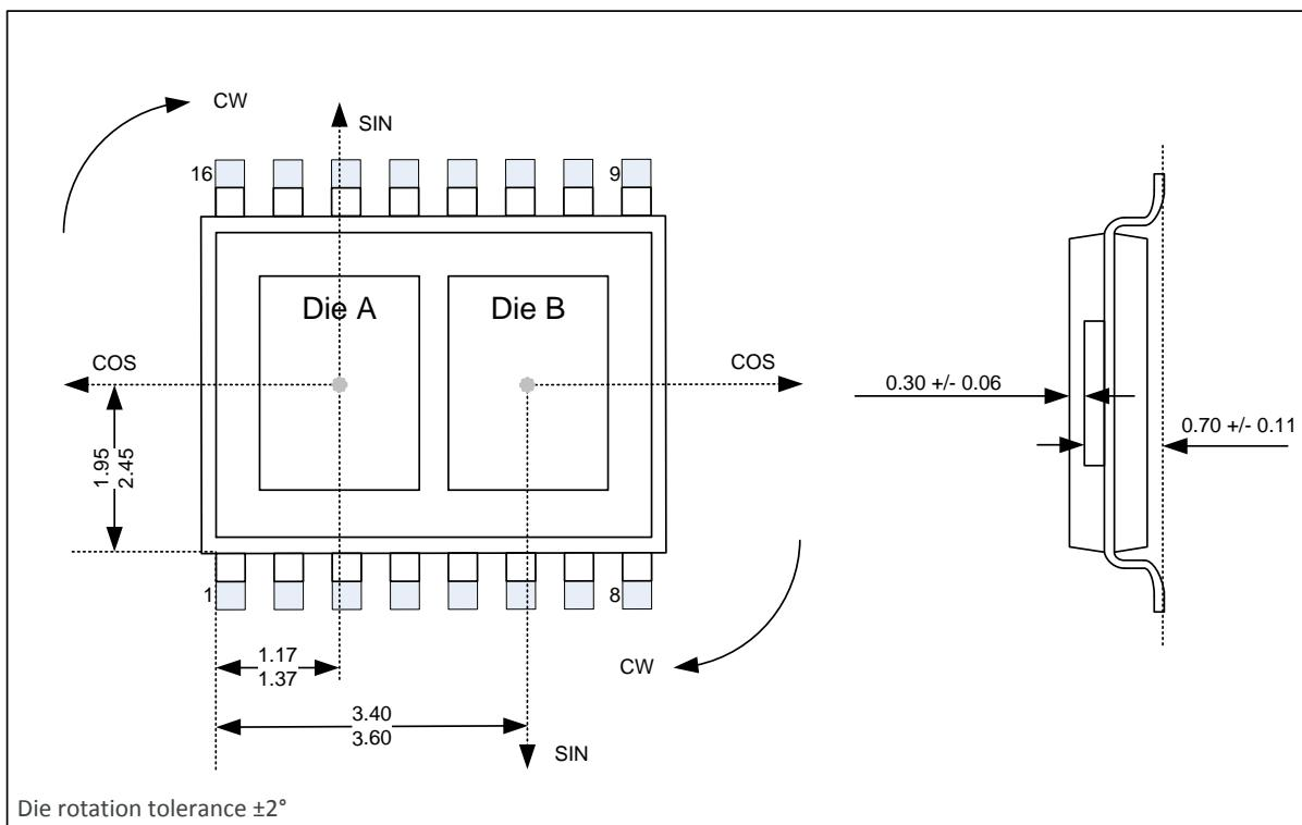
Figure 22: TSSOP-16 IMC positioning
