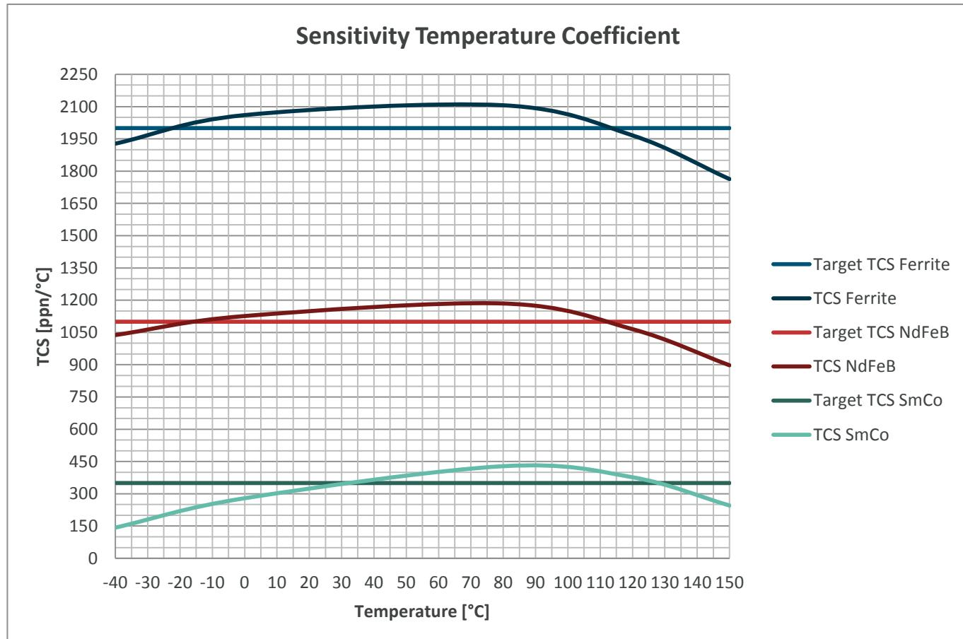
Figure 9: Target TCS vs. 2<sup>nd</sup> order TCS
