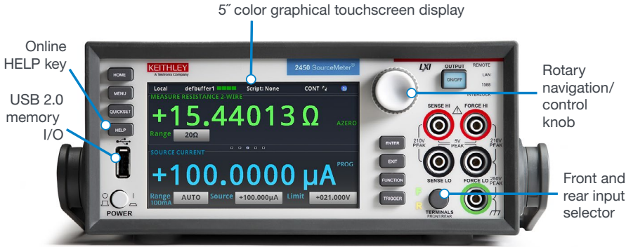
2450 front panel with high-resolution, capacitive touchscreen.
