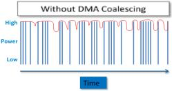
As shown by the red line, components have less time between DMA calls to reach and stay in lower power states.
