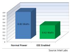
Energy Efficient Ethernet reduces the controller power to approximately 50% of its normal operating level.
