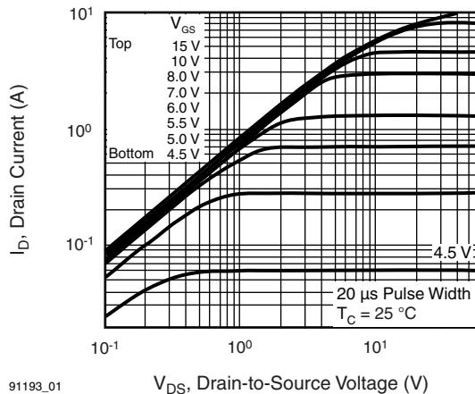
**Fig. 1 - Typical Output Characteristics,  $T_C = 25$  °C**
