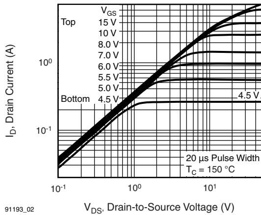
**Fig. 2 - Typical Output Characteristics,  $T_C = 150$  °C**
