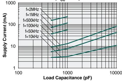
**Supply Current vs. Load Capacitance**
