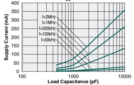
**Supply Current vs. Load Capacitance**
