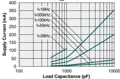
**Supply Current vs. Load Capacitance**
