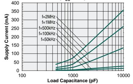
**Supply Current vs. Load Capacitance**
