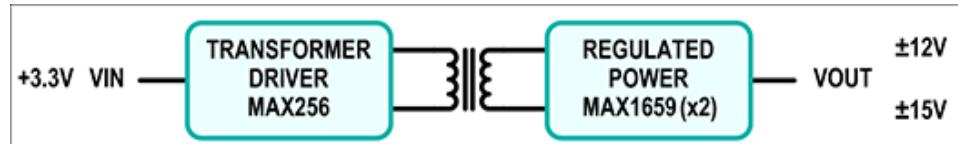
Figure 1. The Lakewood subsystem design block diagram.
