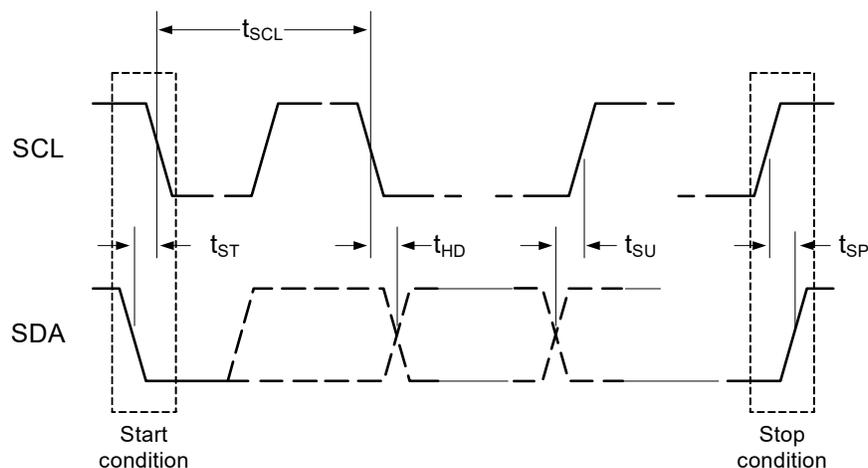
Figure 2: I<sup>2</sup>C Data Transfer
