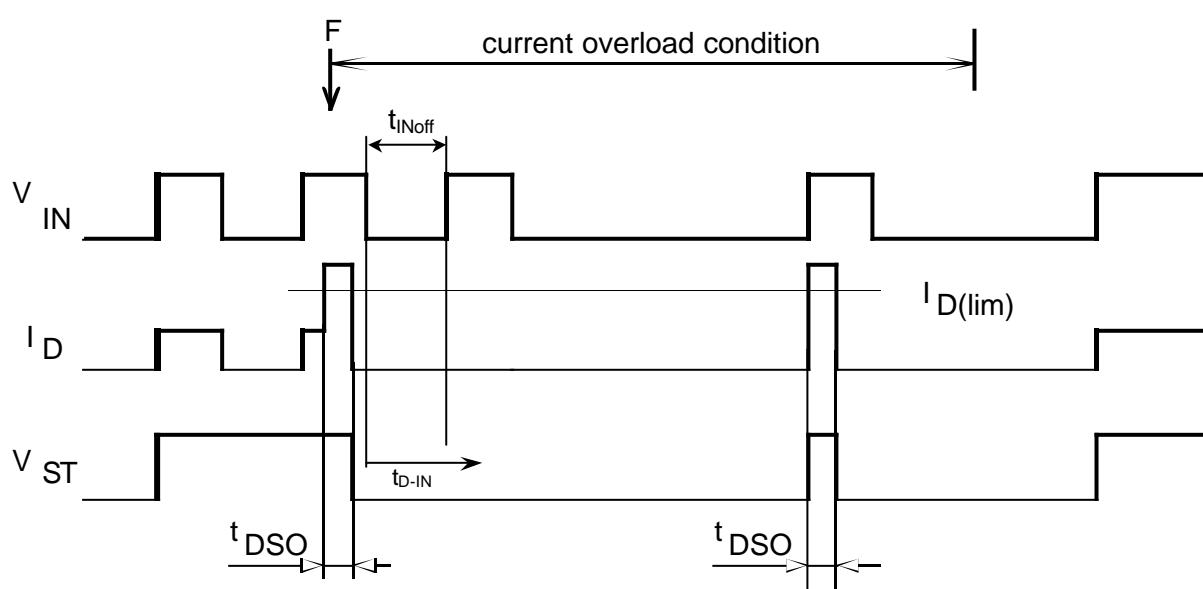
$t_{INoff} < t_{D-IN}$  : Input suppression time avoids a restart after overtemperature
