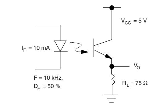
Fig. 10 - Switching Schematic
