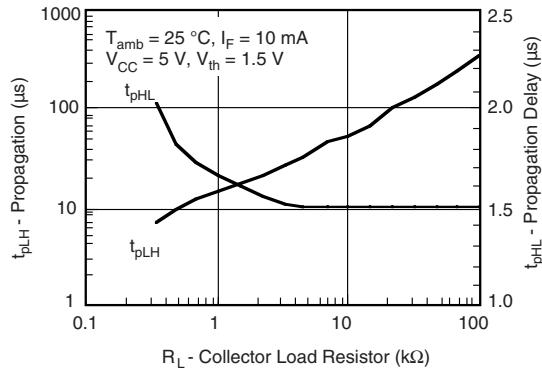
Fig. 8 - Propagation Delay vs. Collector Load Resistor
