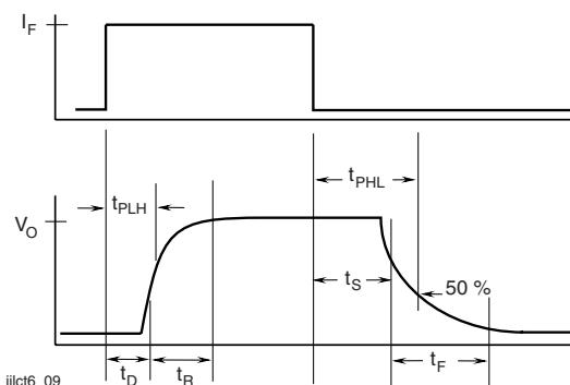
Fig. 9 - Switching Timing
