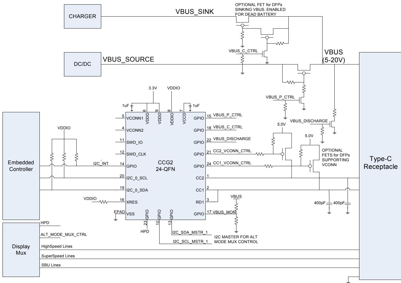
**Figure 11. Downstream Facing Port (DFP) Application**
