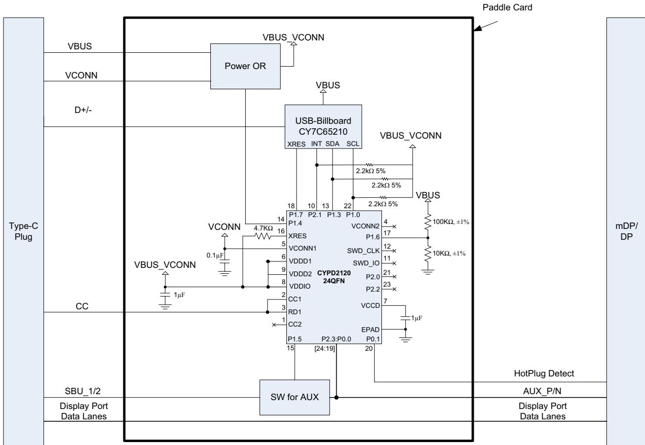
**Figure 14. CCG2 in Dock/Monitor Application Diagram**
