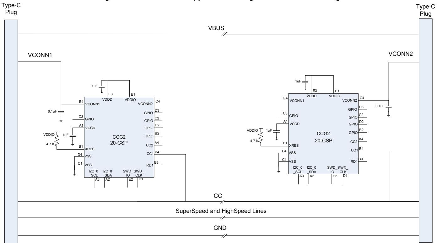
**Figure 9. Upstream Facing Port (UFP) Application – Tablet with a Type-C Port**
