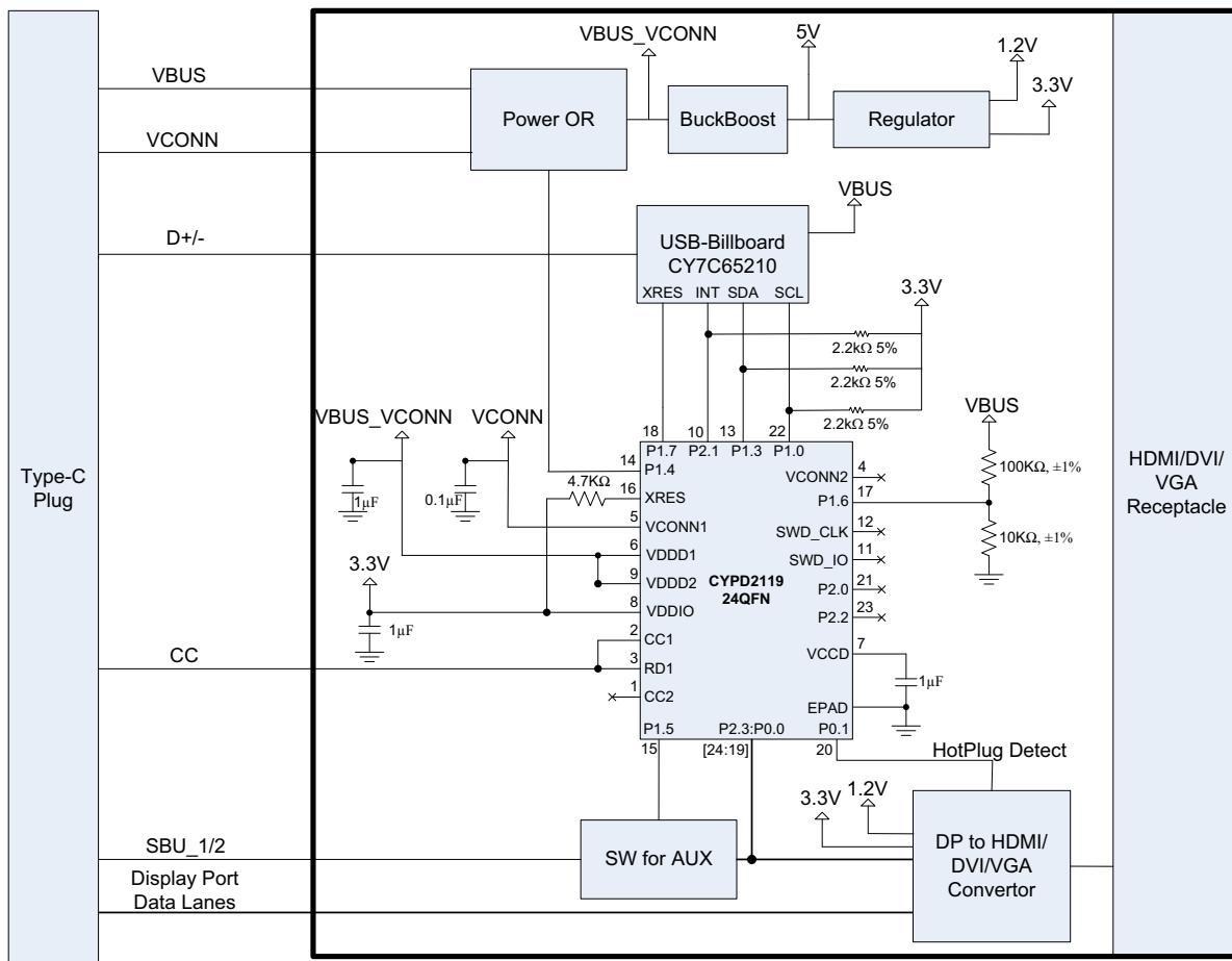
**Figure 13. USB Type-C to Display Port Application Diagram**
