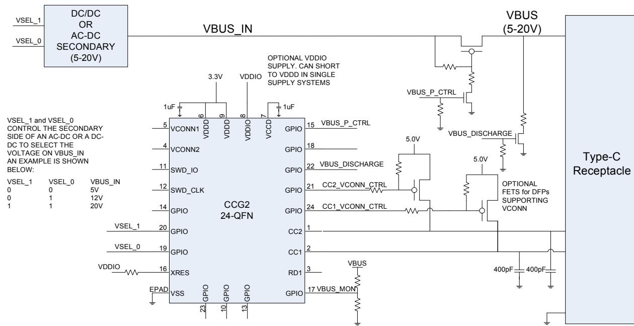
**Figure 12. USB Type-C to HDMI/DVI/VGA Dongle Application Diagram**
