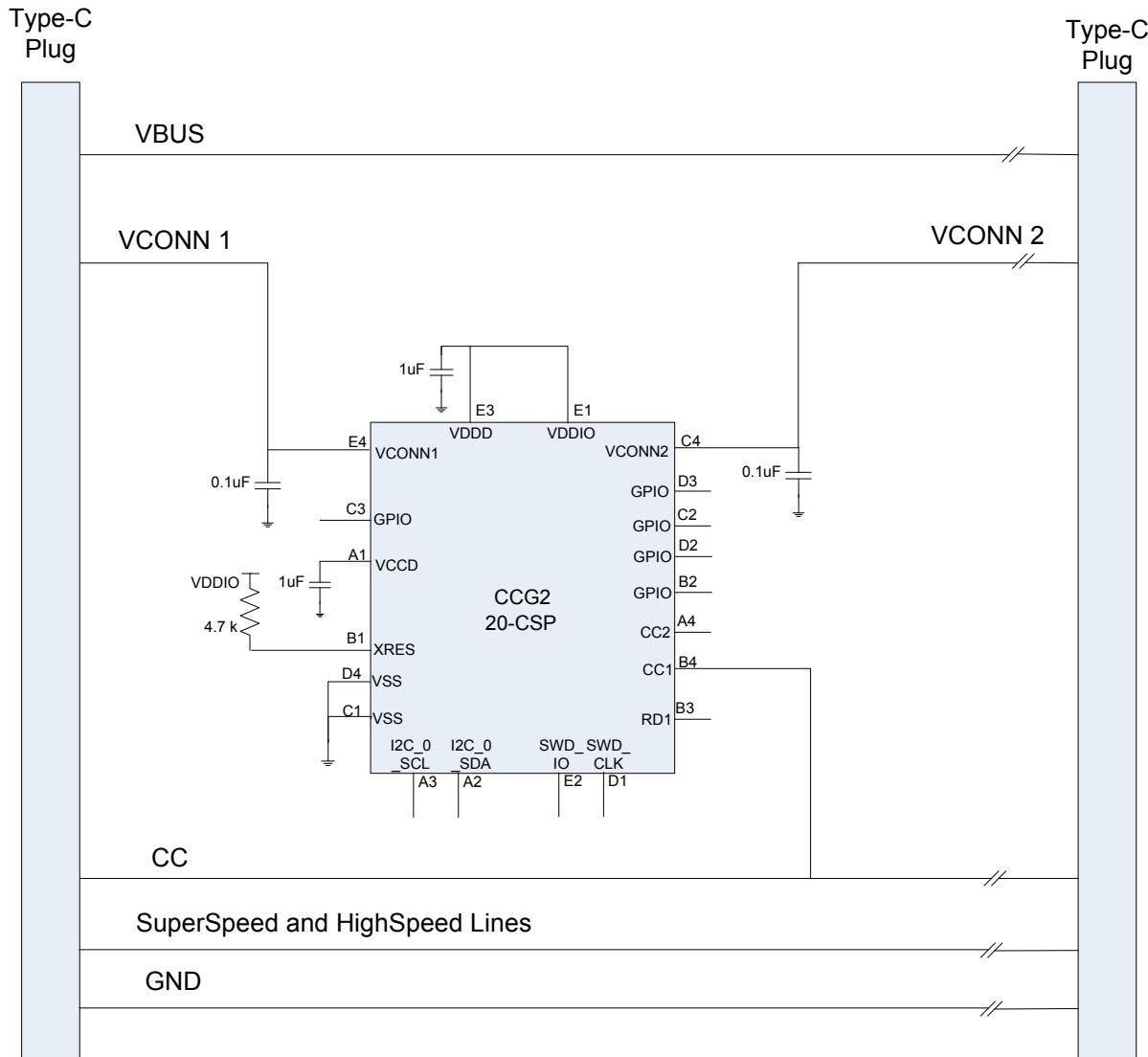
**Figure 8. Passive EMCA Application – Single EZ-PD CCG2 Per Plug**
