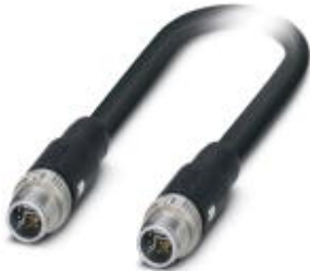
Assembled Ethernet cable, CAT5e, shielded, 8-wire, 4 x 26 AWG (data) and 4 x 20 AWG (power), RAL 9005 (black), M12 hybrid plug to M12 hybrid plug, length: 0.5 m
