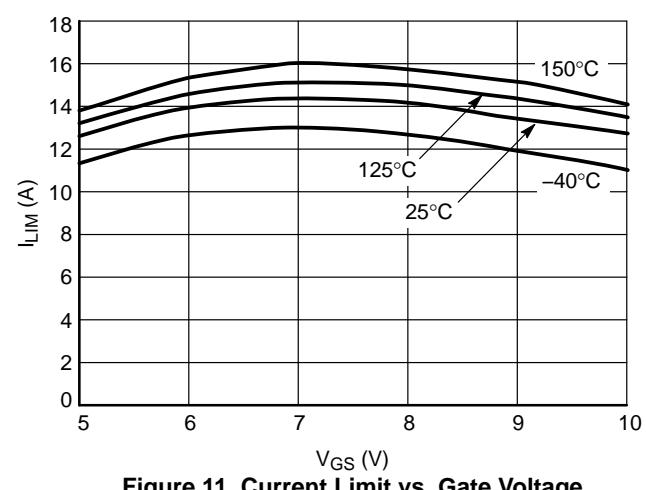
**Figure 11. Current Limit vs. Gate Voltage**
