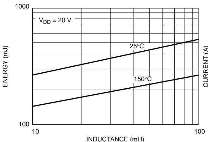
**Figure 8. NCV8408 Maximum Switch Off Energy vs Inductance**
