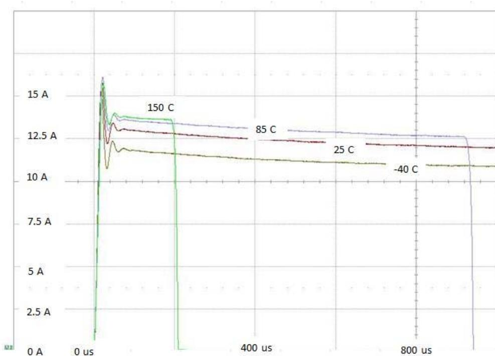
Figure 7. Turn on into Short Circuit Device Response
