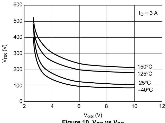
**Figure 10.  $V_{GS}$  vs  $V_{DS}$**
