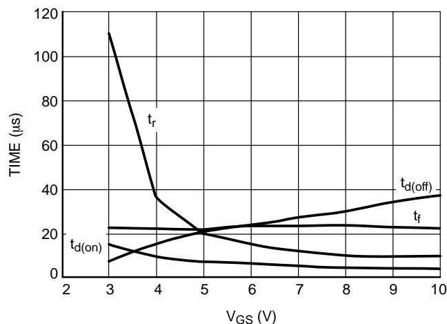
Figure 14. Resistive Switching
