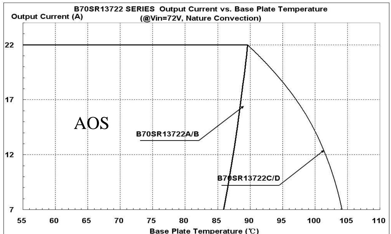
Figure 22: Output Current vs. base plate temperature @ $V_{in}=72V$
