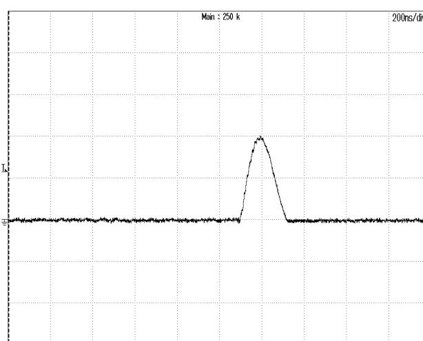
**Figure 11:** Inrush current @ Vin=72V
