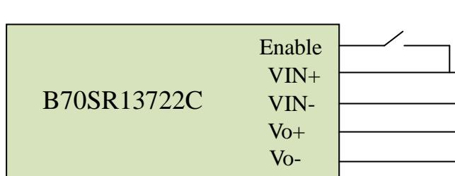
*Figure 12: suggested Enable connection*
