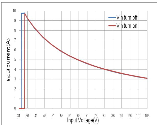
**Figure 7:** Input current vs. Input voltage
