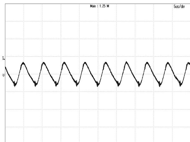
**Figure 5:** Output ripple & noise at 72Vin, 22A lout
