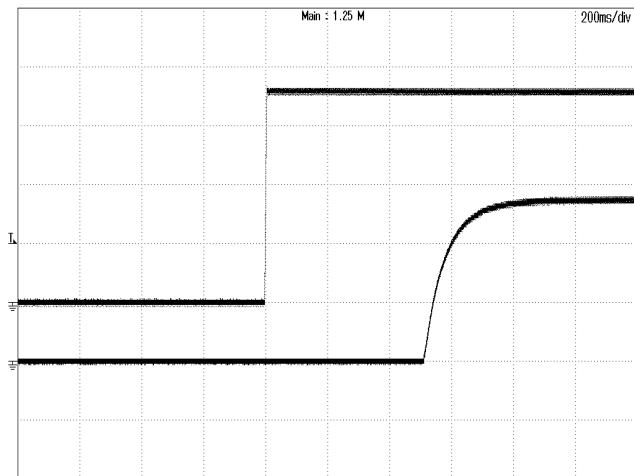
**Figure 4:** Vout start up with Vin on at 72Vin, 22A lout,
