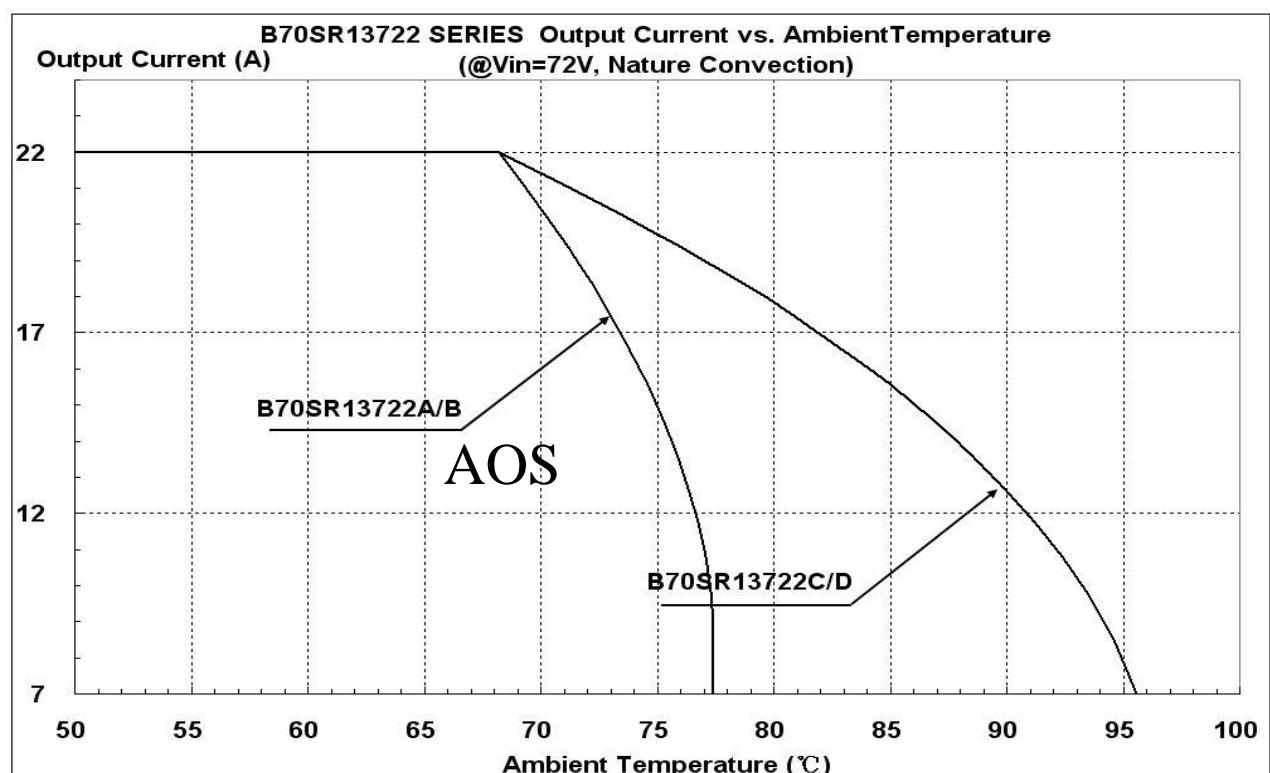
Figure 18: Output Current vs. ambient temperature @ $V_{in}=72V$
