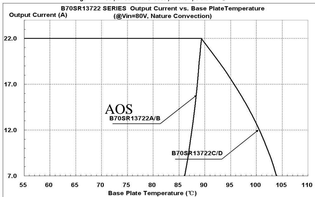
Figure 23: Output Current vs. base plate temperature @ $V_{in}=80V$
