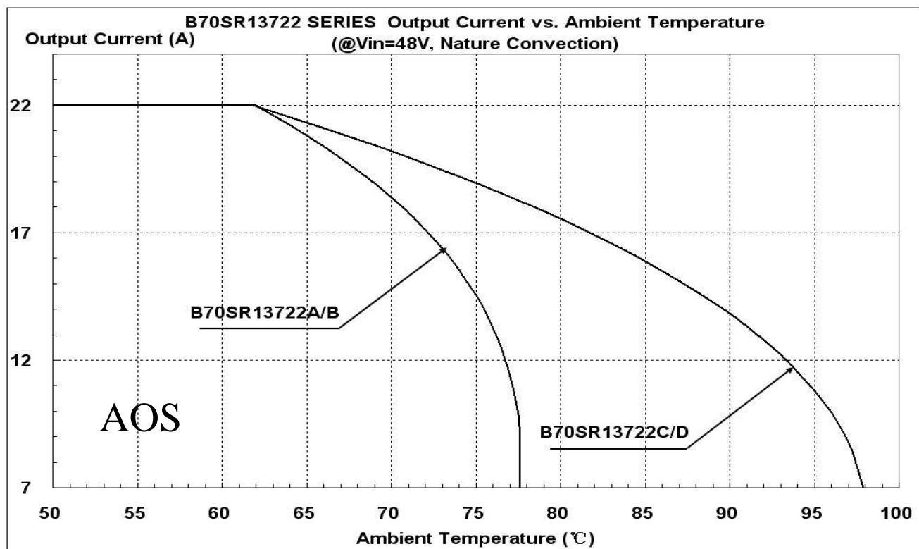
Figure 17: Output Current vs. ambient temperature @Vin=48V
