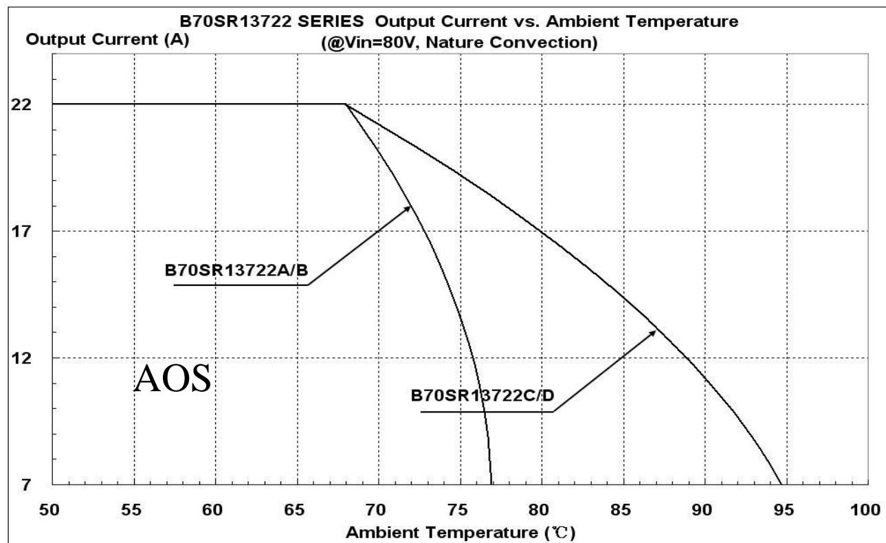
Figure 19: Output Current vs. ambient temperature @ $V_{in}=80V$
