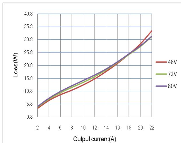
**Figure 2:** Loss vs. Output current
