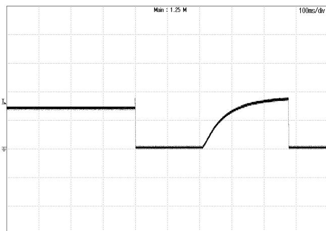
**Figure 6:** Output over voltage protection at 72Vin, 22A lout
