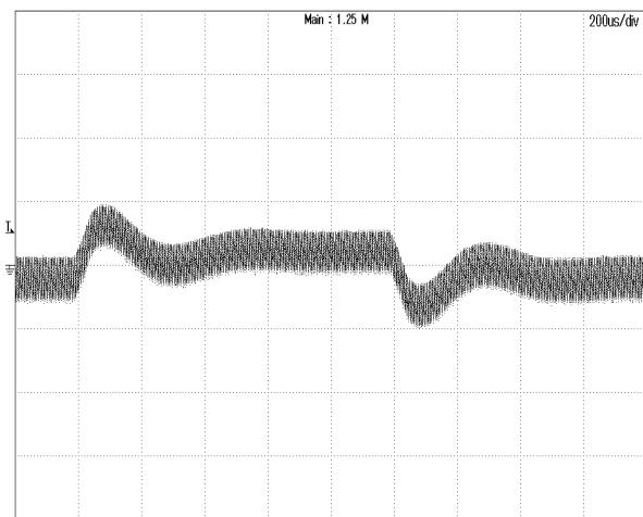
**Figure 3:** Dynamic response to load step 11A~16.5A with 0.1A/uS slew rate at 72Vin
