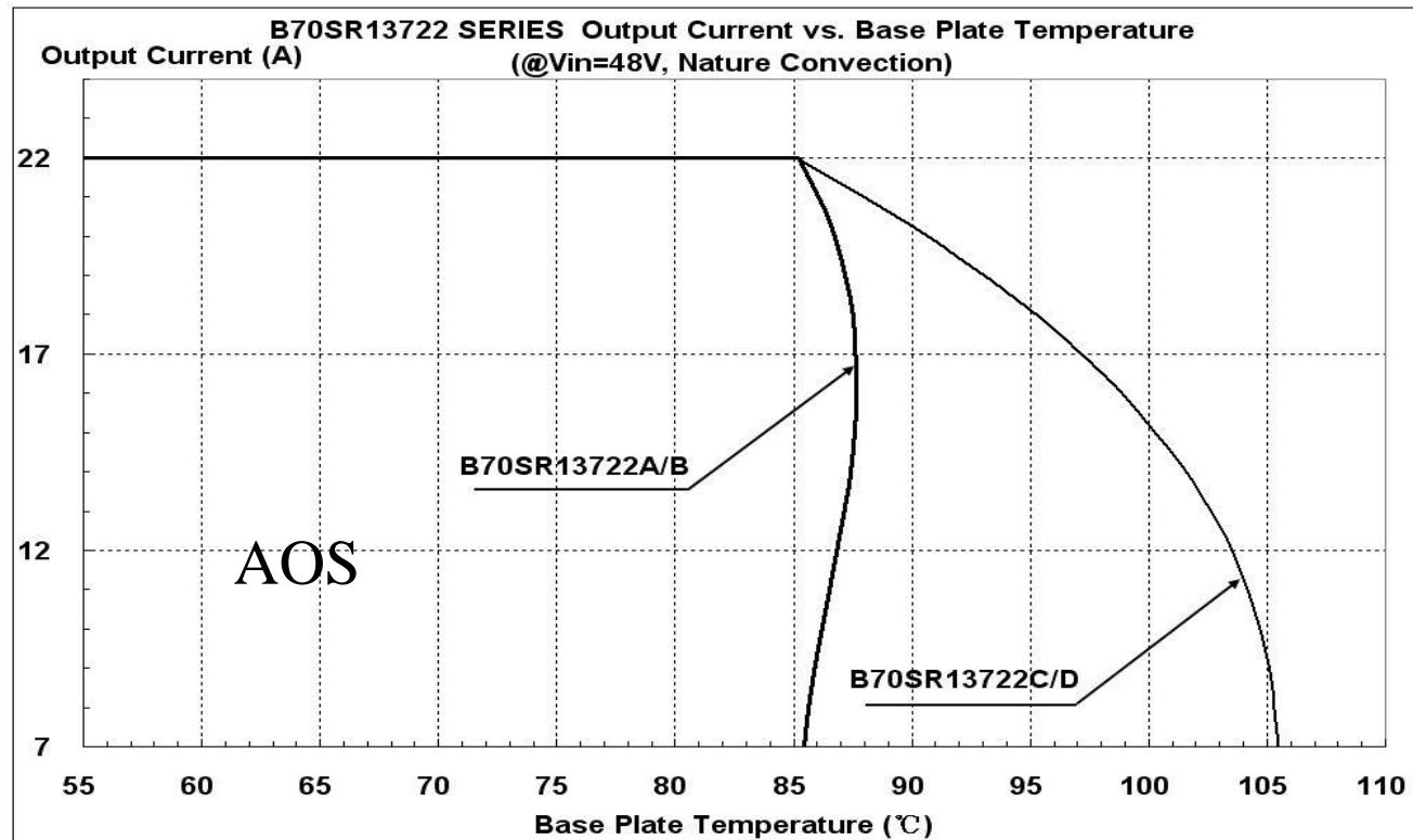
Figure 21: Output Current vs. base plate temperature @Vin=48V
