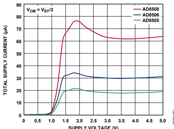
Figure 21. Total Supply Current vs. Supply Voltage
