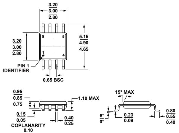
Figure 53. 8-Lead Mini Small Outline Package [MSOP]
