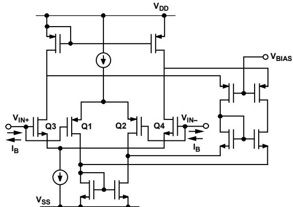
Figure 45. A Typical Dual Differential Pair Input Stage Op Amp
