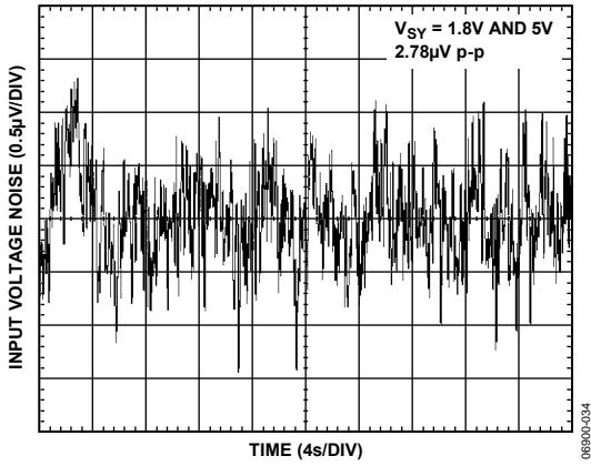
Figure 39. Input Voltage Noise 0.1 Hz to 10 Hz
