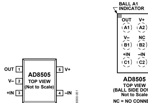
Figure 1. 5-Lead SOT-23 (RJ-5)
