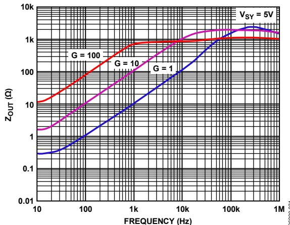
Figure 30.  $Z_{\text{OUT}}$  vs. Frequency
