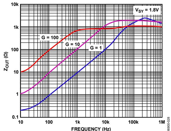
Figure 27.  $Z_{\text{OUT}}$  vs. Frequency
