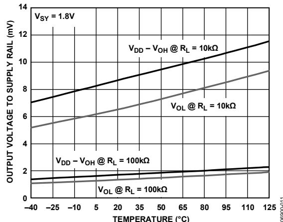
Figure 20. Output Voltage to Supply Rail vs. Temperature
