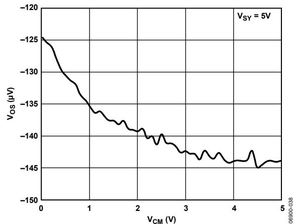
Figure 16. Input Offset Voltage vs. Input Common-Mode Voltage
