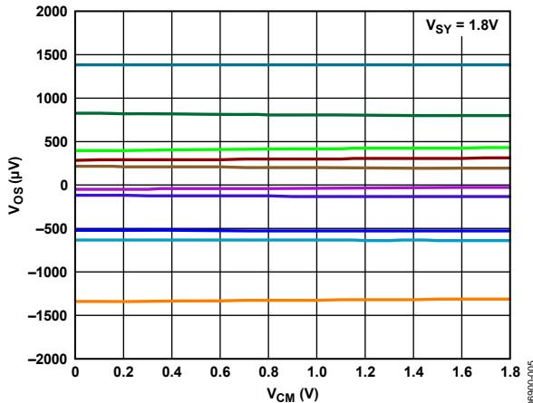
Figure 9. Input Offset Voltage vs. Input Common-Mode Voltage
