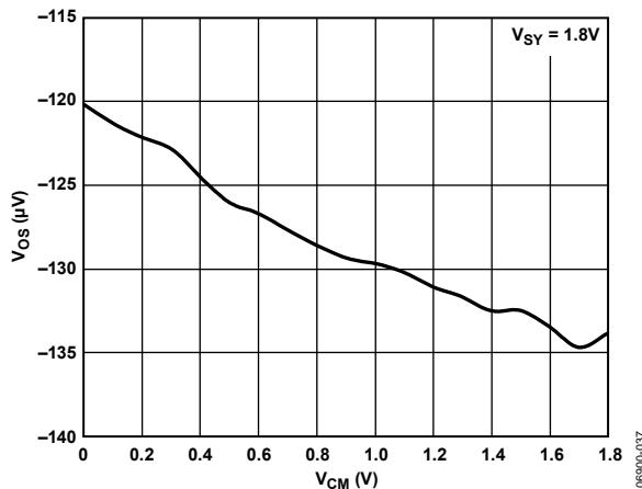
Figure 13. Input Offset Voltage vs. Input Common-Mode Voltage
