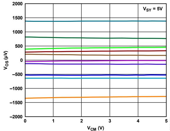
Figure 12. Input Offset Voltage vs. Input Common-Mode Voltage
