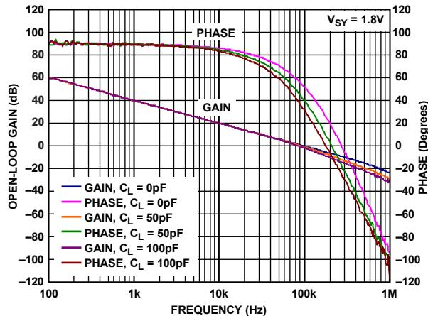
Figure 25. Open-Loop Gain and Phase vs. Frequency
