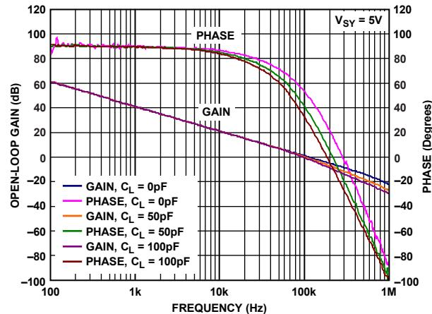
Figure 28. Open-Loop Gain and Phase vs. Frequency
