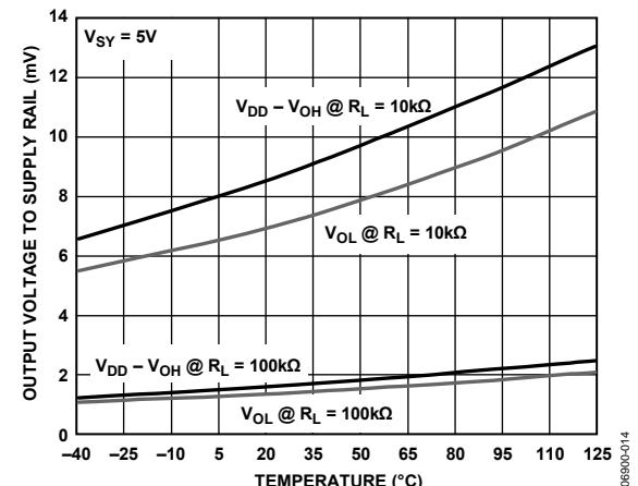
Figure 23. Output Voltage to Supply Rail vs. Temperature
