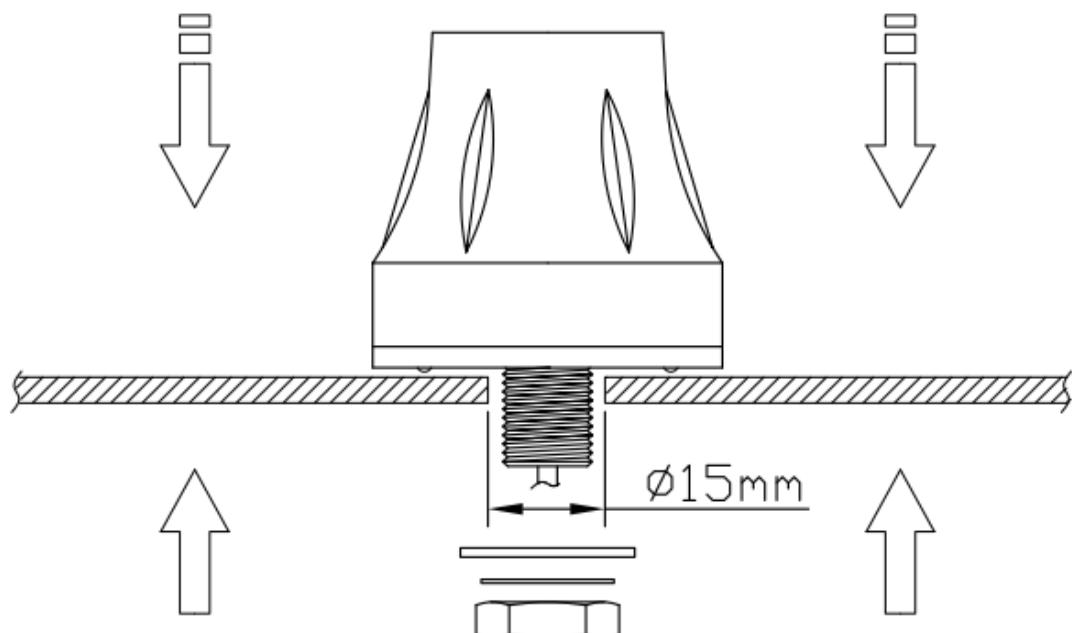
Recommended torque for mounting is 2.94N.m
