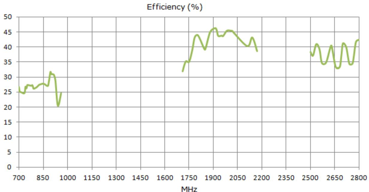
**Figure 6.** Efficiency of G30 Antenna in Free Space
