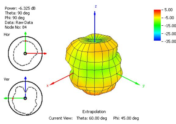
**Figure 27.** Radiation Pattern at 751MHz of G30 Antenna on 30\*30cm metal
