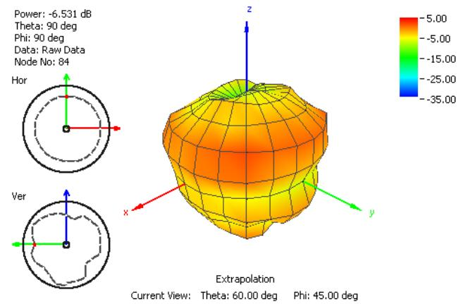
**Figure 31.** Radiation Pattern at 1805MHz of G30 Antenna on 30\*30cm metal.
