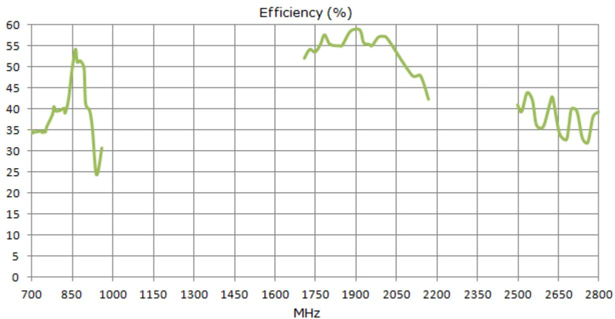
**Figure 7.** Efficiency of G30 Antenna on 30x30cm metal
