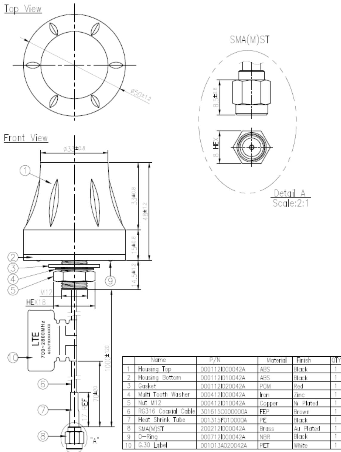
Figure 37. Mechanical Drawing of the G30 Antenna
