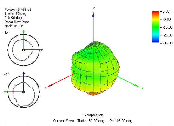
**Figure 19.** Radiation Pattern at 849MHz of G30 Antenna in Free Space
