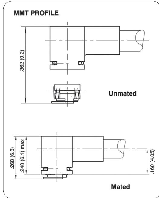
RADIALl has designed a complete range of microminiature coaxial connectors, dedicated to **Surface Technology (SMT)**.
