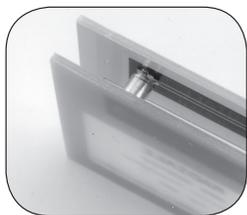
To ease PCB linking, this adapter is designed to remain mated to one designated PCB. Therefore, the slit interface is slide-on, the other is snap-on. This adapter can also be developed upon request with other lengths, in order to adjust space between PCB (minimum distance: 6.4 mm). Please consult us.
