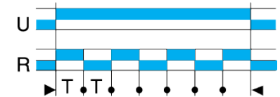
Function Di: Symmetrical flashing
