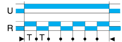
Function Di: Symmetrical flashing
