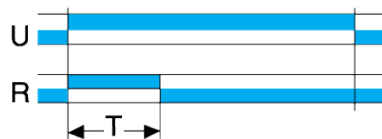
Function H: Timing on energization – Pulse output (adjustable)
